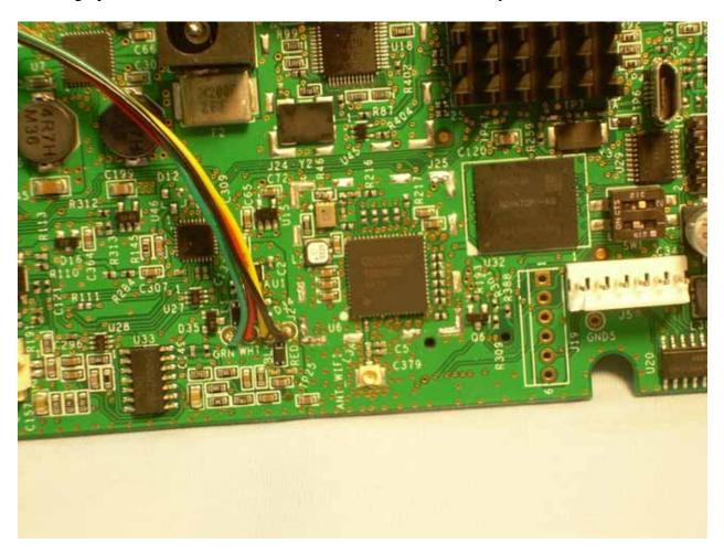
Photograph 11 – View of the Back Side of the Main PCB Circuitry with RF Shield Removed
