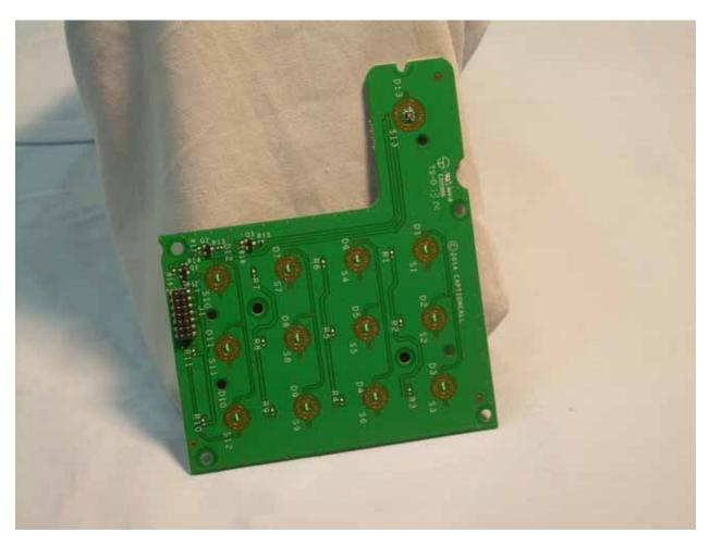
Photograph 16 – View of the Front Side of the Button Interface PCB
