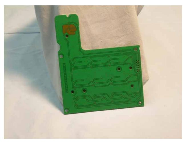
Photograph 17 – View of the Back Side of the Button Interface PCB
