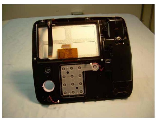
Photograph 19 - Internal View of the EUT with PCBs Removed
