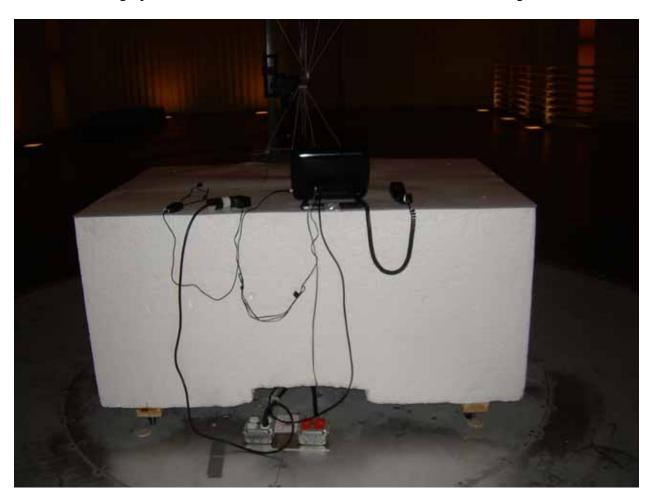
Photograph 2 – Back View Radiated Disturbance Worst Case Configuration
