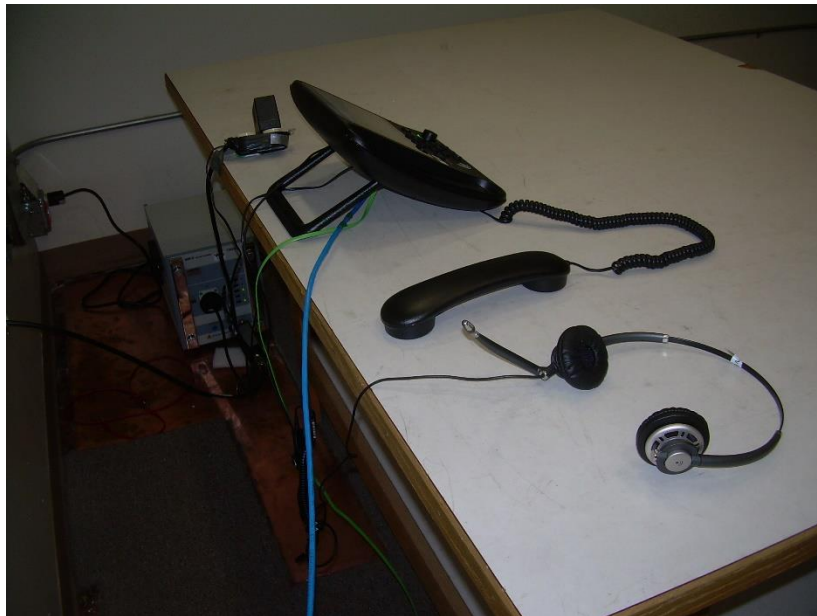
Photograph 2: Back View Conducted Emissions Worst-Case Configuration
