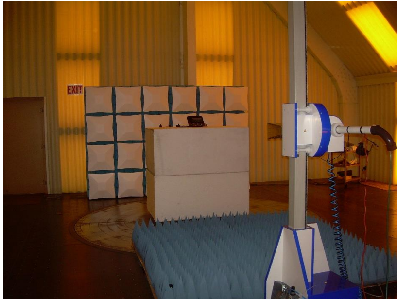
Photograph 5 – Front View Radiated Emissions Worst-Case Configuration – Above 1000 MHz
