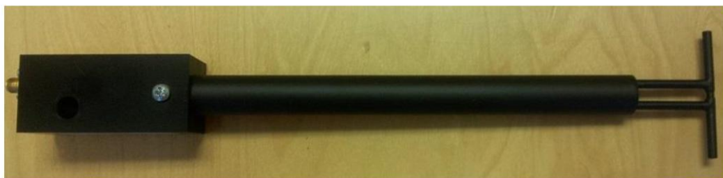
Figure 1 – MVG COMOSAR Validation Dipole
