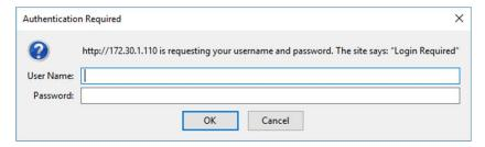
The default User Name is "admin" and the default password is the serial number (S/N) printed on the bottom of the gateway. For security, you should change the password using the Security tab after logging in.
