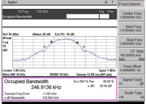
Occupied Bandwidth (99%) GPRS 1900 BAND CH 810
