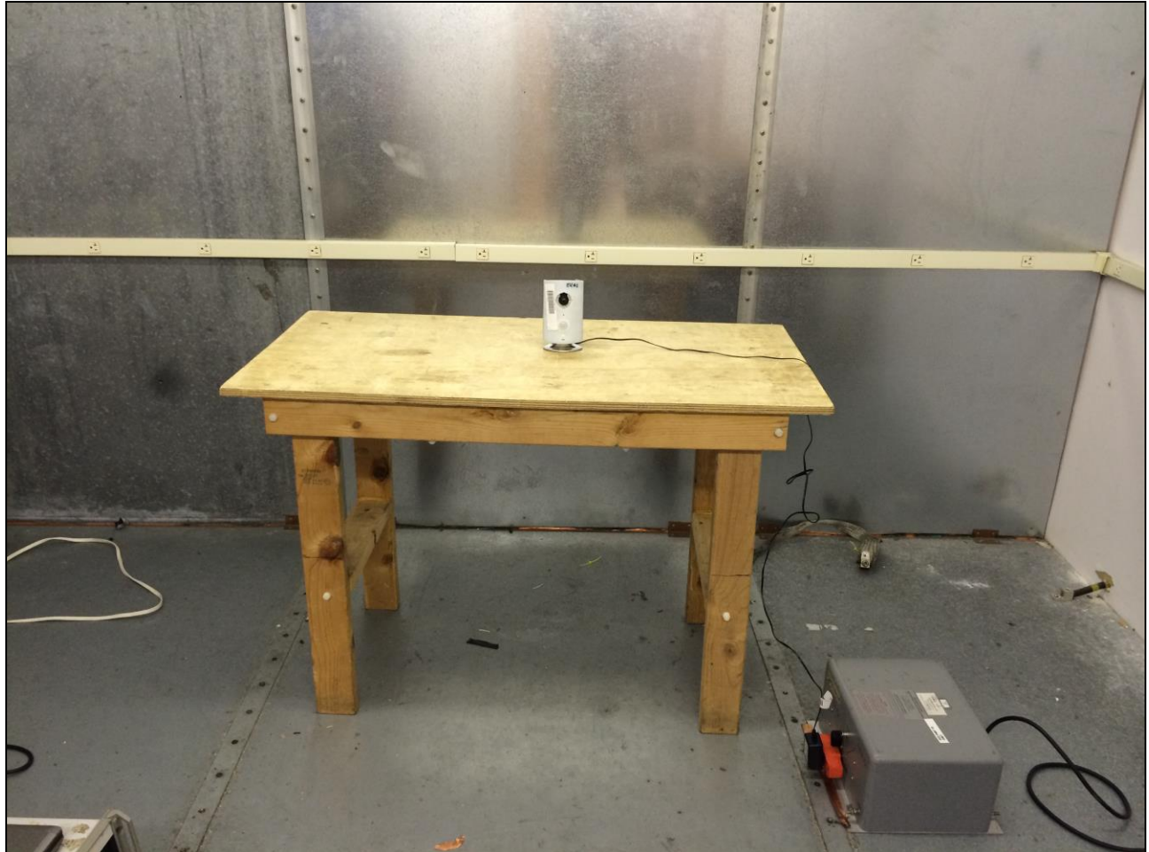
Photograph 3. Conducted Emissions, 15.207(a), Test Setup
