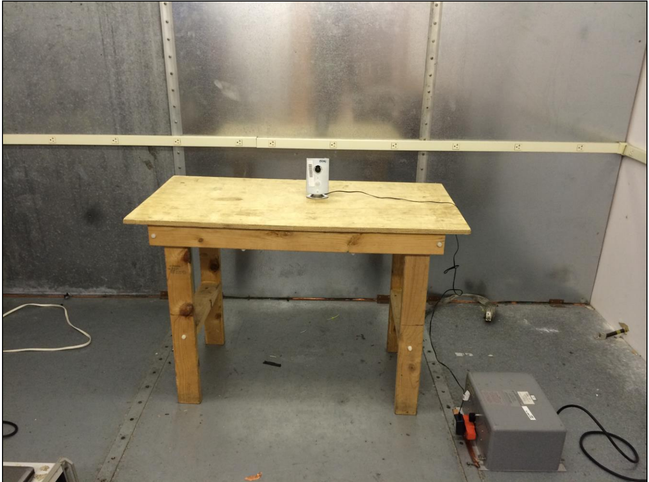
Photograph 1. Conducted Emissions, Test Setup
