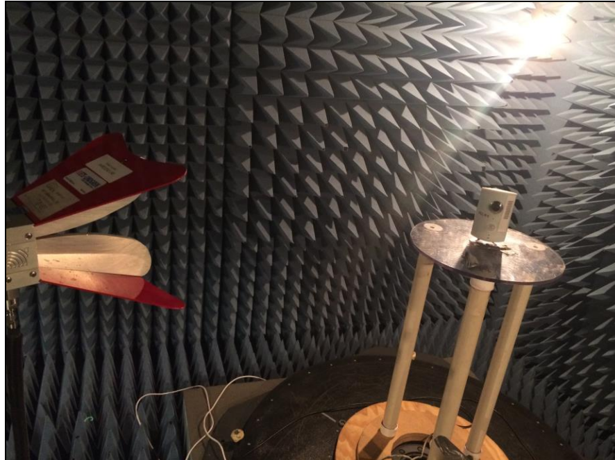
Photograph 5. Radiated Spurious Emissions, Test Setup, Above 1 GHz
