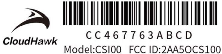
Specifications: Text is black in color and justified. Labels are printed in indelible ink on permanent adhesive silk-screened onto the EUT or shall be affixed at a conspicuous location on the EUT.
