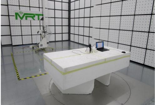
Test Mode: Mode 1/ Mode 2/ Mode 3 Description: Radiated Emission Test Setup for above 1GHz
