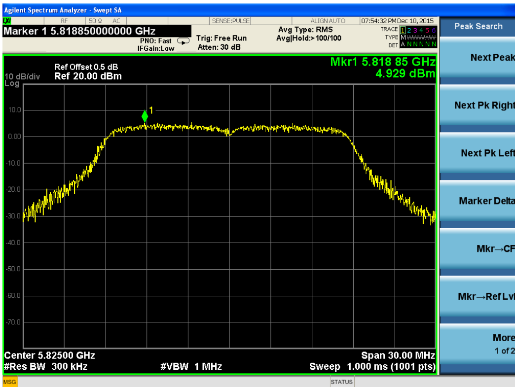
Test Plot For 802.11n(HT20)-5825M-Chain 1
