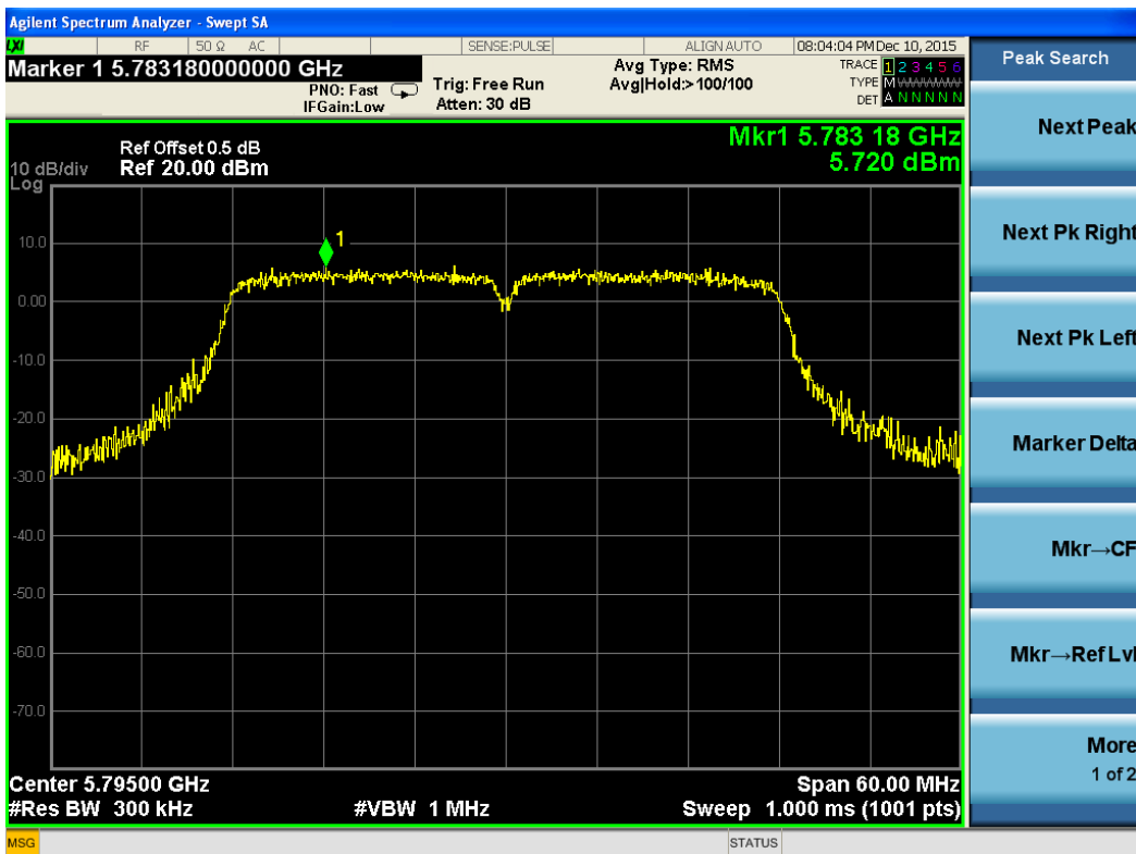
Test Plot For 802.11n(HT40)-5795M-Chain 1
