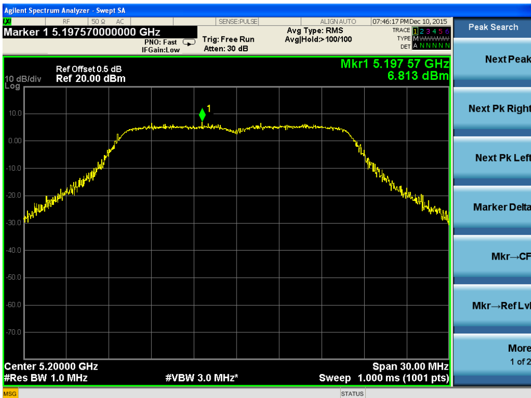
Test Plot For 802.11a-5200M-Chain 1
