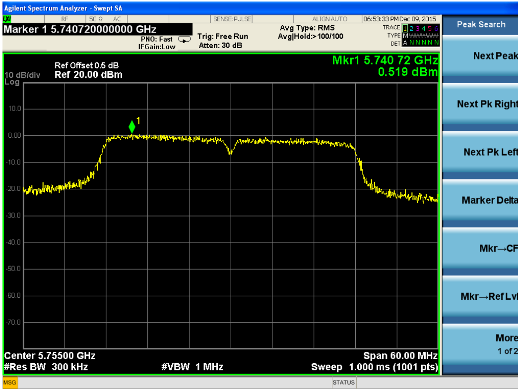
Test Plot For 802.11n(HT40)-5755M-Chain 2
