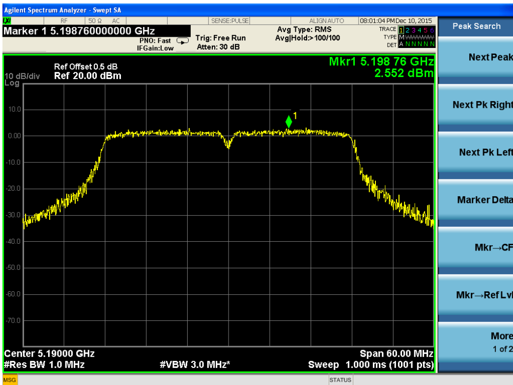
Test Plot For 802.11n(HT40)-5190M-Chain 1
