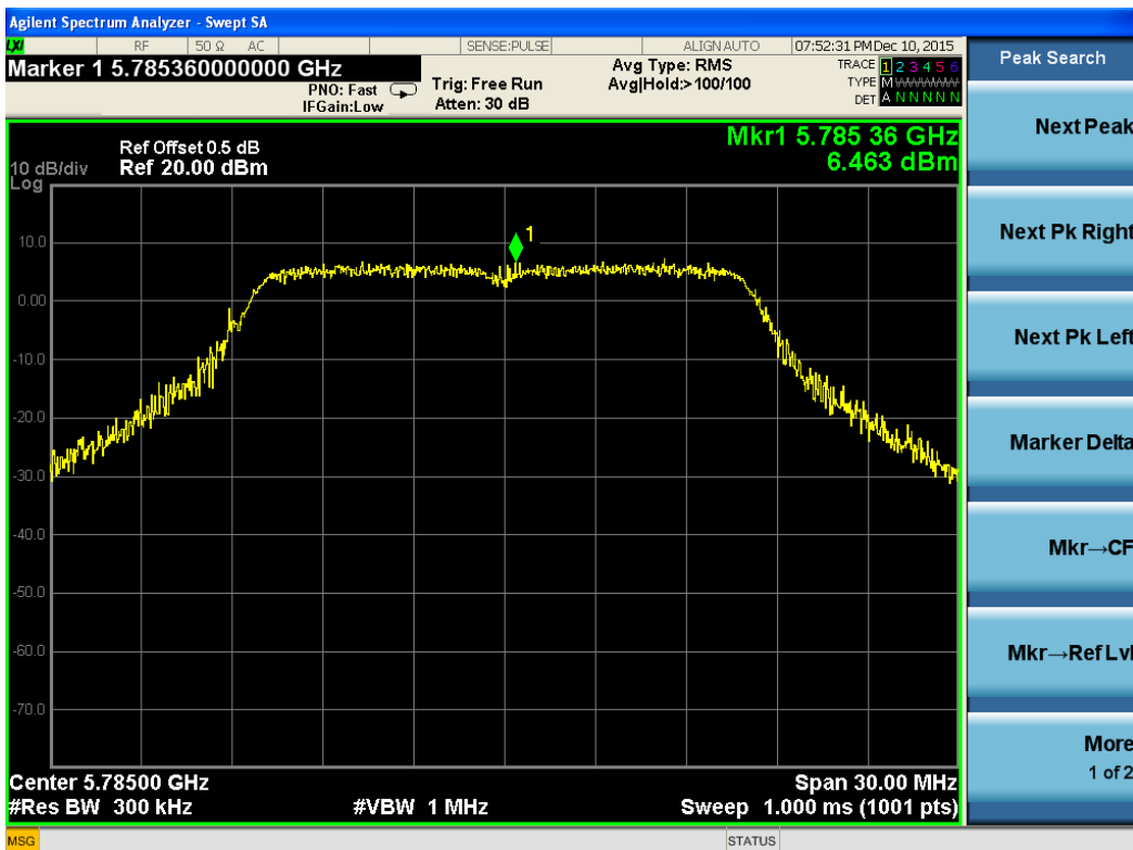
Test Plot For 802.11a-5785M-Chain 3
