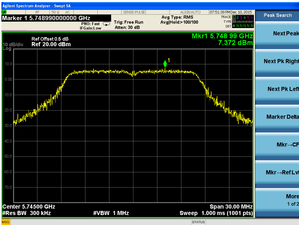
Test Plot For 802.11a-5745M-Chain 3
