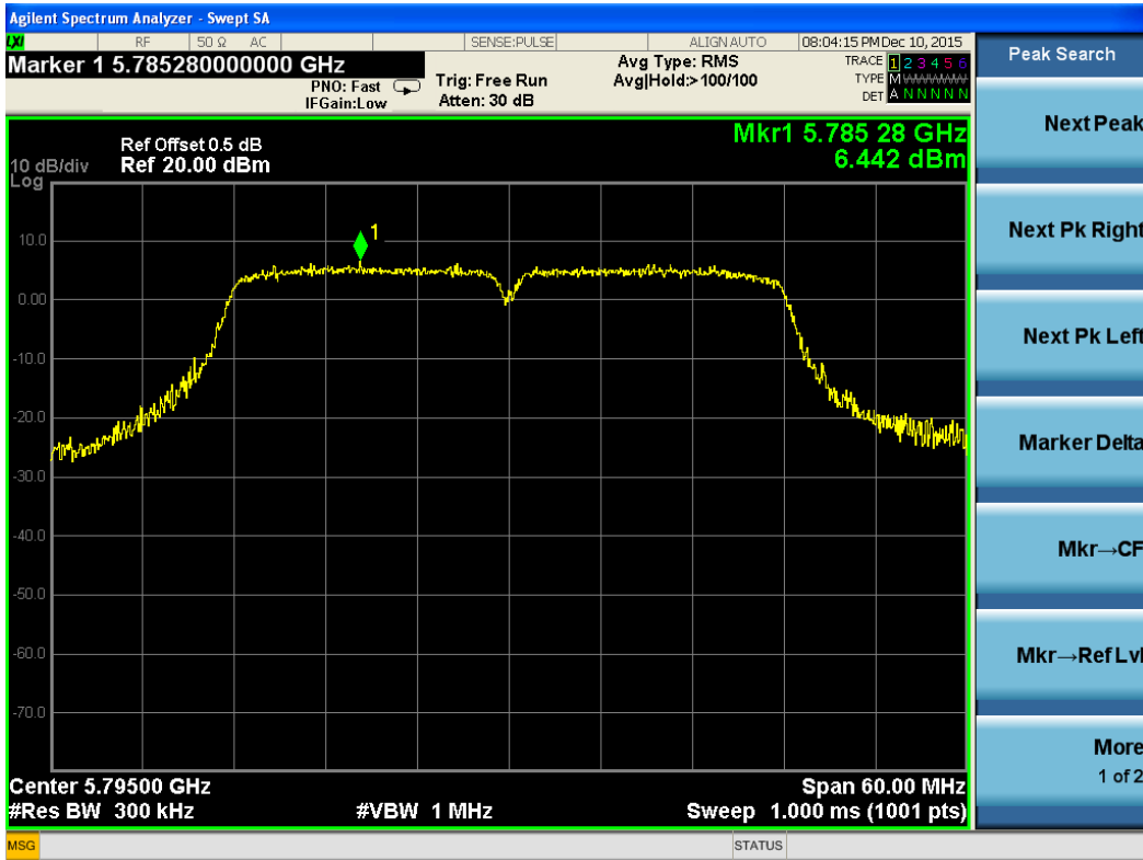
Test Plot For 802.11n(HT40)-5795M-Chain 0
