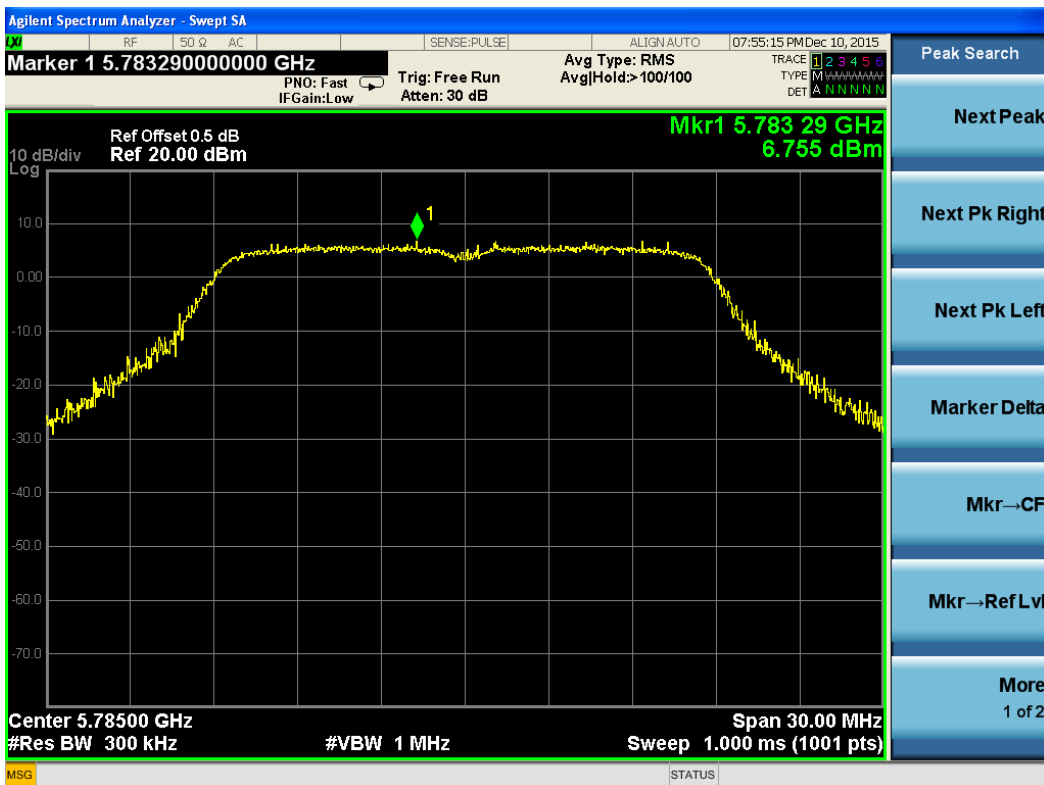
Test Plot For 802.11n(HT20)-5785M-Chain 1
