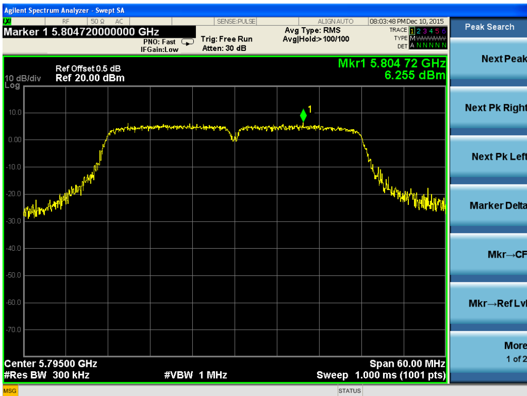
Test Plot For 802.11n(HT40)-5795M-Chain 3
