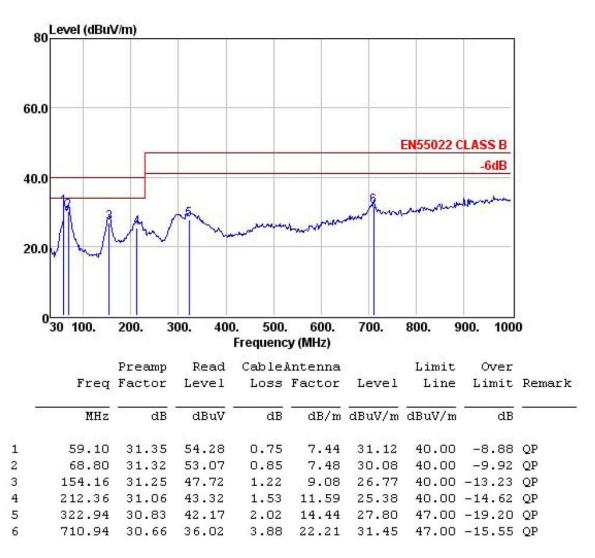
Test mode: TX Mode Polarization: HORIZONTAL
