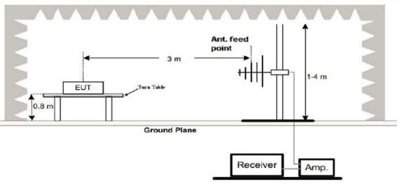
(3) Radiated Emission Test-Up Frequency Above 1GHz
