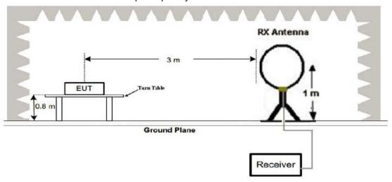
(2) Radiated Emission Test-Up Frequency 30MHz~1GHz
