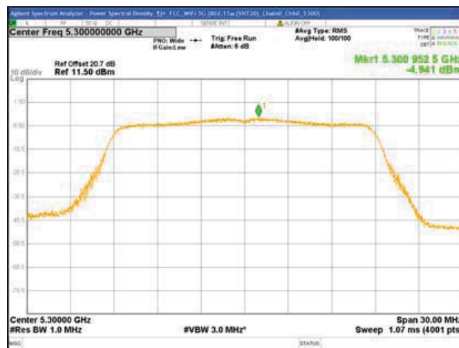
Chain0 : Power Spectral Density @ 802.11ac(VHT20) Mode Ch64
