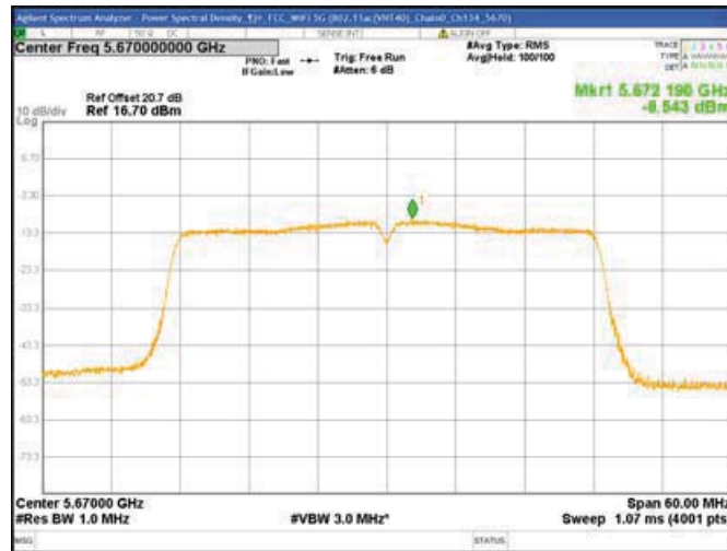
Chain0 : Power Spectral Density @ 802.11ac(VHT40) Mode Ch151
