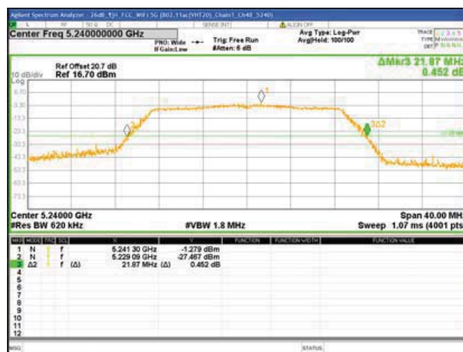
Chain1 : 26dB Bandwidth @ 802.11ac(VHT20) Mode Ch48
