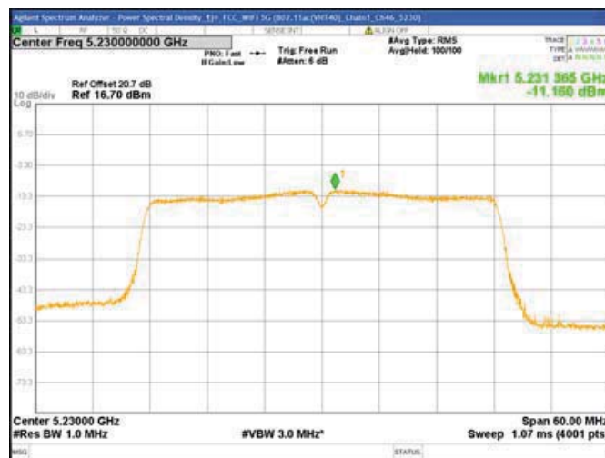
Chain1 : Power Spectral Density @ 802.11ac(VHT40) Mode Ch54
