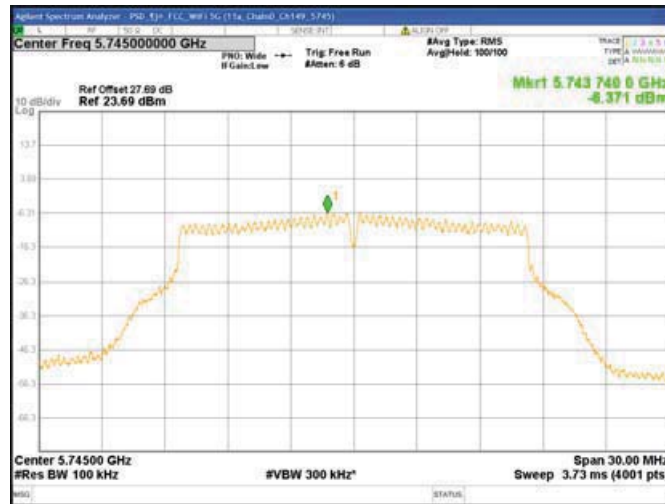
Chain0 : Power Spectral Density @ 802.11a Mode Ch157
