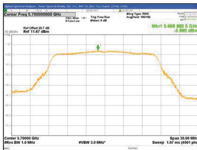
Chain0 : Power Spectral Density @ 802.11a Mode Ch140
