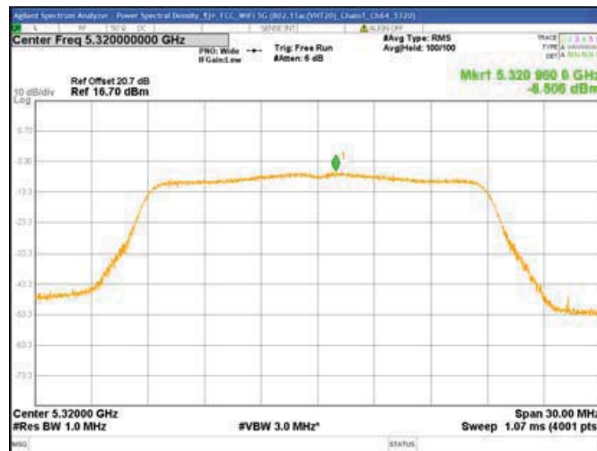
Chain1 : Power Spectral Density @ 802.11ac(VHT20) Mode Ch64
