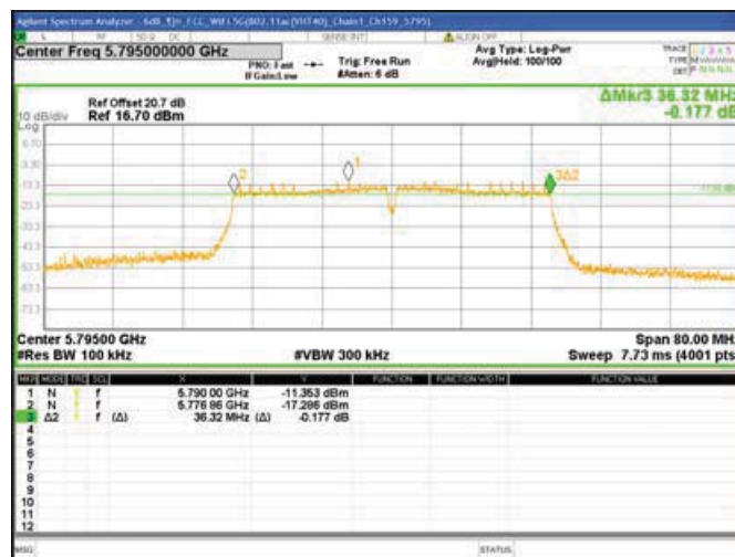
Chain0 : 6dB Bandwidth @ 802.11ac(VHT80) Mode Ch122
