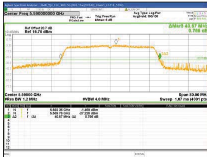
Chain1 : 26dB Bandwidth @ 802.11ac(VHT40) Mode Ch134
