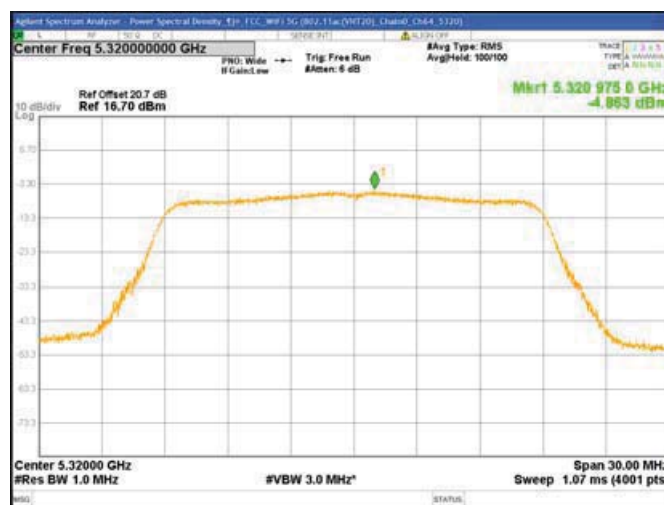
Chain0 : Power Spectral Density @ 802.11ac(VHT20) Mode Ch64
