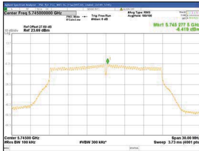
Chain0 : Power Spectral Density @ 802.11ac(VHT20) Mode Ch157
