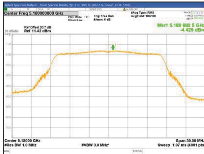
Chain1 : Power Spectral Density @ 802.11a Mode Ch44
