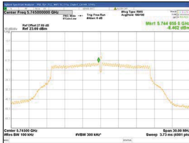
Chain 1 : Power Spectral Density @ 802.11a Mode Ch157
