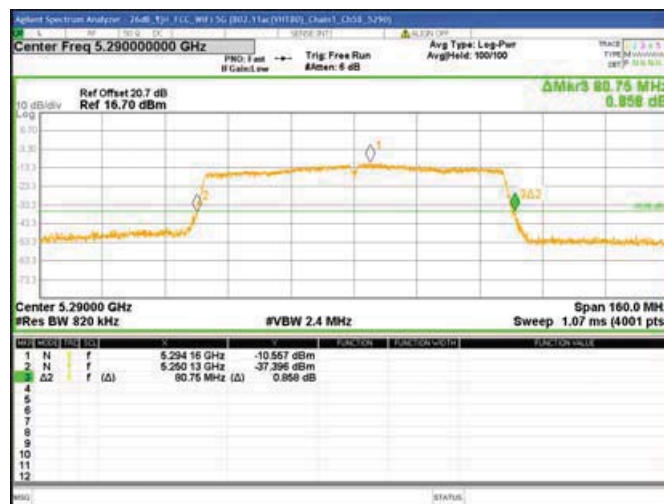
Chain1 : 26dB Bandwidth @ 802.11ac(VHT80) Mode Ch106
