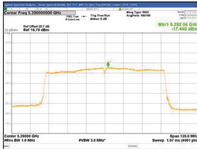
Chain1 : Power Spectral Density @ 802.11ac(VHT80) Mode Ch106
