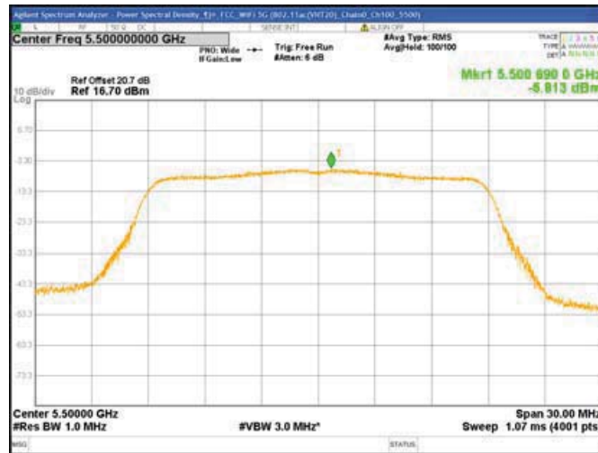
Chain0 : Power Spectral Density @ 802.11ac(VHT20) Mode Ch120
