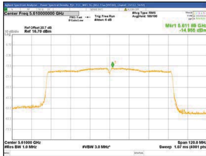
Chain0 : Power Spectral Density @ 802.11ac(VHT80) Mode Ch155
