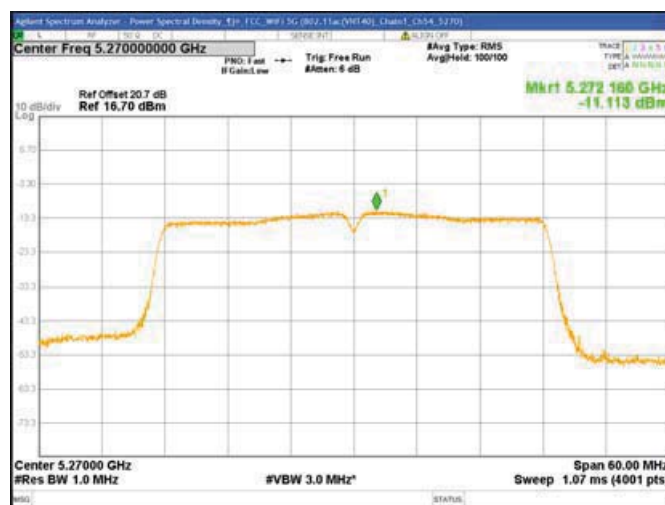
Chain1 : Power Spectral Density @ 802.11ac(VHT40) Mode Ch54
