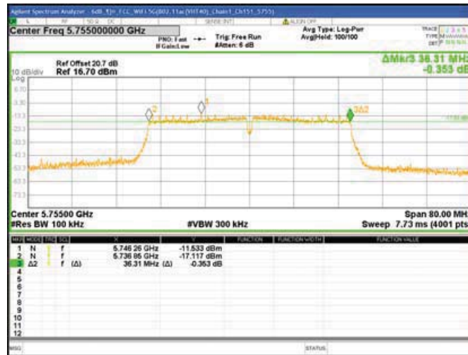
Chain1 : 6dB Bandwidth @ 802.11ac(VHT40) Mode Ch159
