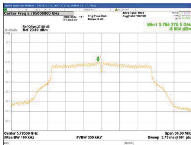
Chain0 : Power Spectral Density @ 802.11a Mode Ch165
