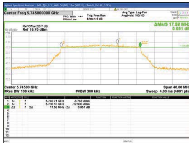
Chain0 : 6dB Bandwidth @ 802.11ac(VHT20) Mode Ch157
