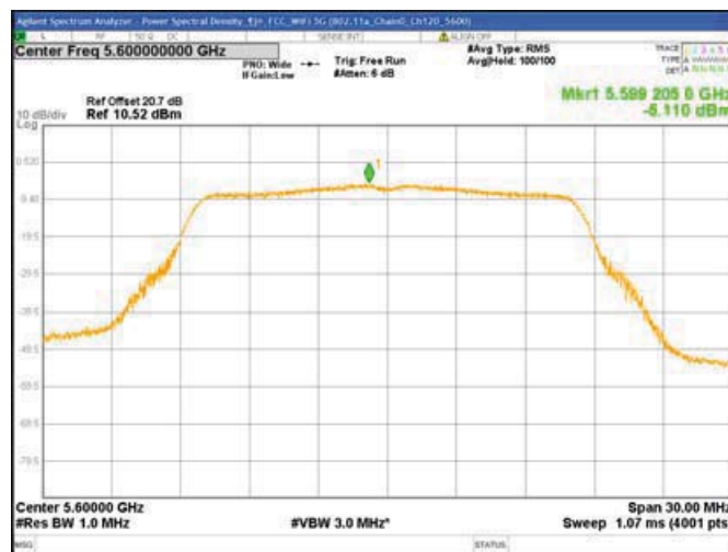
Chain0 : Power Spectral Density @ 802.11a Mode Ch140
