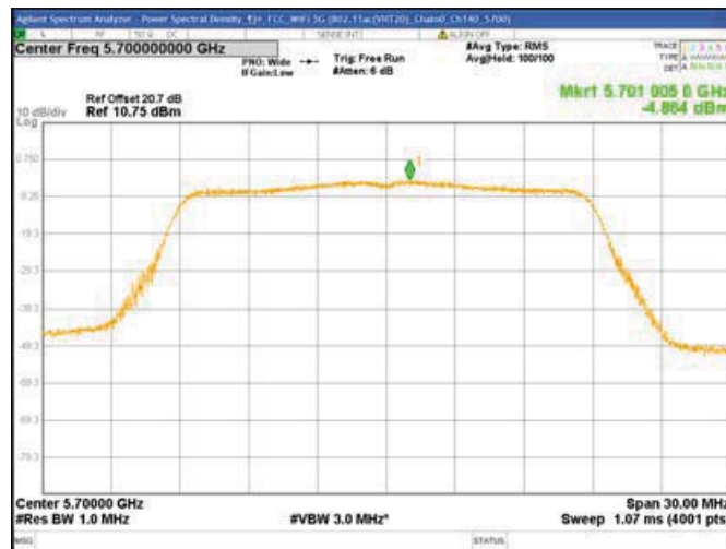
Chain0 : Power Spectral Density @ 802.11ac(VHT20) Mode Ch140
