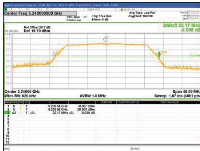
Chain0 : 26dB Bandwidth @ 802.11ac(VHT20) Mode Ch48
