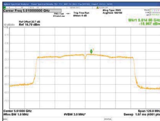
Chain1 : Power Spectral Density @ 802.11ac(VHT80) Mode Ch122
