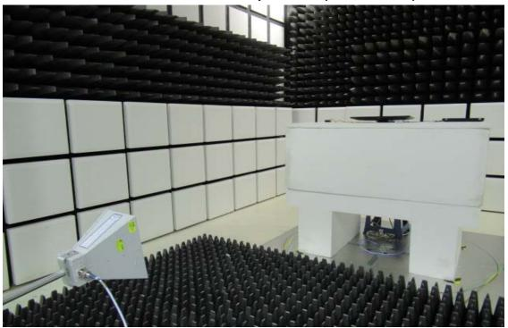
Radiated Emission Set up Photos (Front View)
