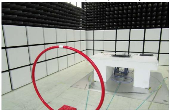
Radiated Emission Set up Photos (Below 1GHz)
