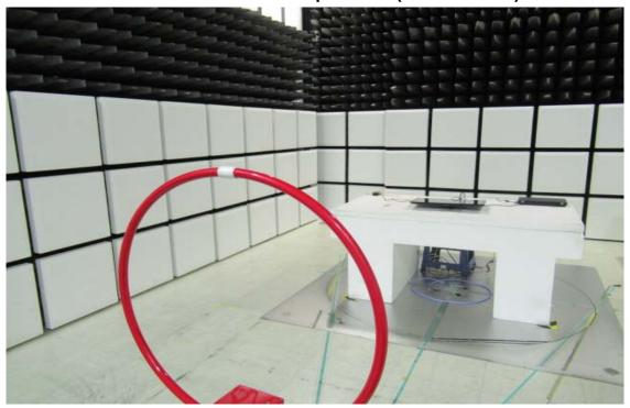
Radiated Emission Set up Photos (Below 1GHz)
