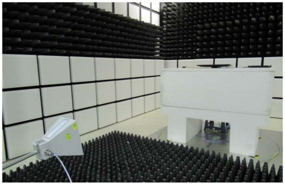
Radiated Emission Set up Photos (Front View)
