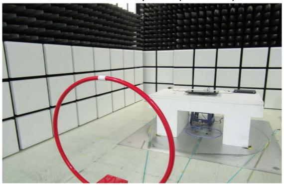
Radiated Emission Set up Photos (Below 1GHz)
