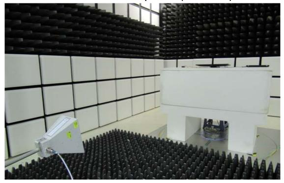
Radiated Emission Set up Photos (Front View)
