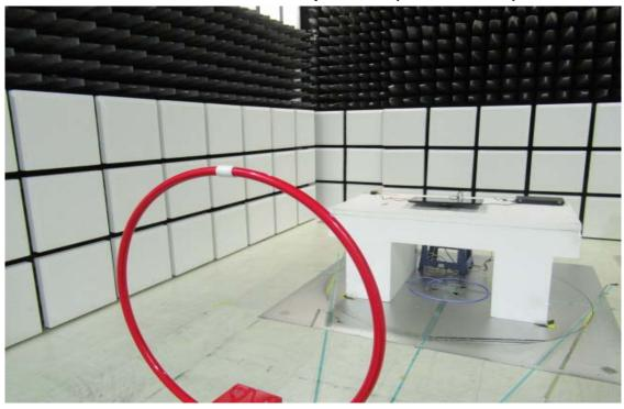
Radiated Emission Set up Photos (Below 1GHz)
