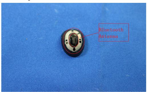
The antenna is integrated on the main PCB and no consideration of replacement. The best case gain of the antenna is -0.6dBi.
