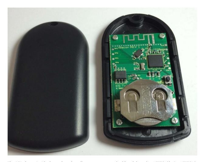
The PCB shown inside the package has all components attached (model number KST3013). For KST3010, KST3011, and KST3012, we simply do not load U2, R2, R3, and R4. You can see these components on the board. We noted these as "NO PLACE" on our BOM.
