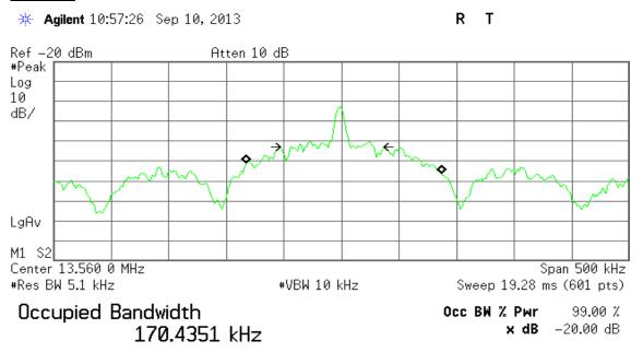
Transmit Freq Error 2.237 kHz x dB Bandwidth 72.825 kHz
