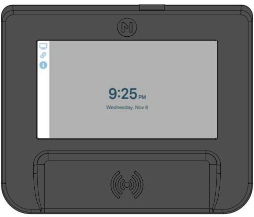
2 Touch the top "Display" icon and then touch Rotate option to rotate the screen 180° for wall mounting.
