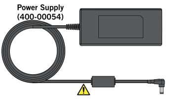
Use only provided AC/DC adapter model W&T-AD36W052300F manufactured by W&T Electronics Co., Ltd., with output rating 5.2VDC @ 3A, or model CDS015-T051, manufactured by Adapter Technology Co., Ltd., with output rating 5.15VDC @ 3A.
