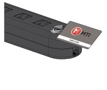
**1b** From an Alarming state, place the User Key over the RFID icon to silence the alarm. Then hold down the User Key for 5 seconds to return back to the disarmed state. LED will be flashing white.
