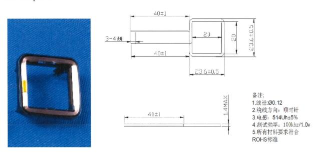
Antenna transmission frequency: 100 – 300kHz
