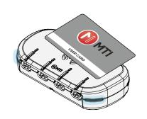
To close Enrollment mode, place the Authorization Card over the RFID icon. Enrollment mode will end automatically after 3 minutes of no use. LED will then be intermittently flashing white.
