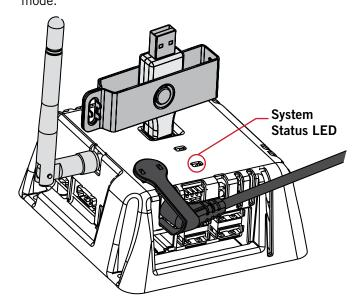
The MTI Connect® Hub will automatically exit pairing mode after 15 minutes and it's status LED will return to the previous state.
