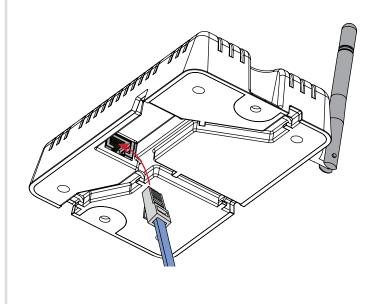
4 Mount the extender using the 3.5 mm x 16 mm screws (or longer if needed) for the mounting surface (not included).
