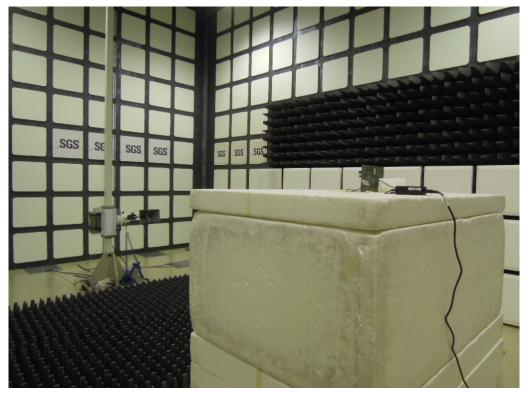
Radiated Emission Set up Photos (Front View)
