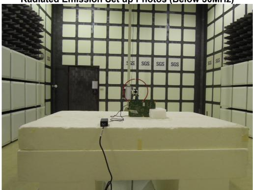
Radiated Emission Set up Photos (Below 1GHz)
