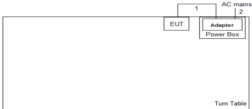
Test Setup Diagram – AC Line Conducted Emission Test
