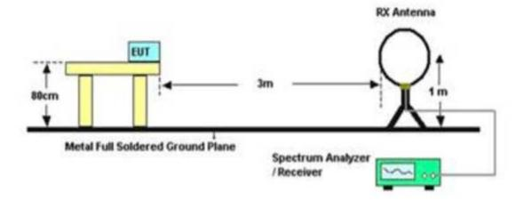
(B) Radiated Emission Test-Up Frequency 30MHz~1GHz
