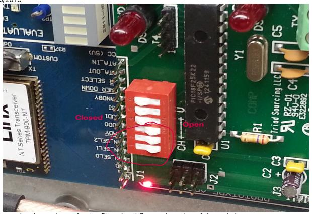
Refer to the above picture for the Closed and Open orientation of the switches.
