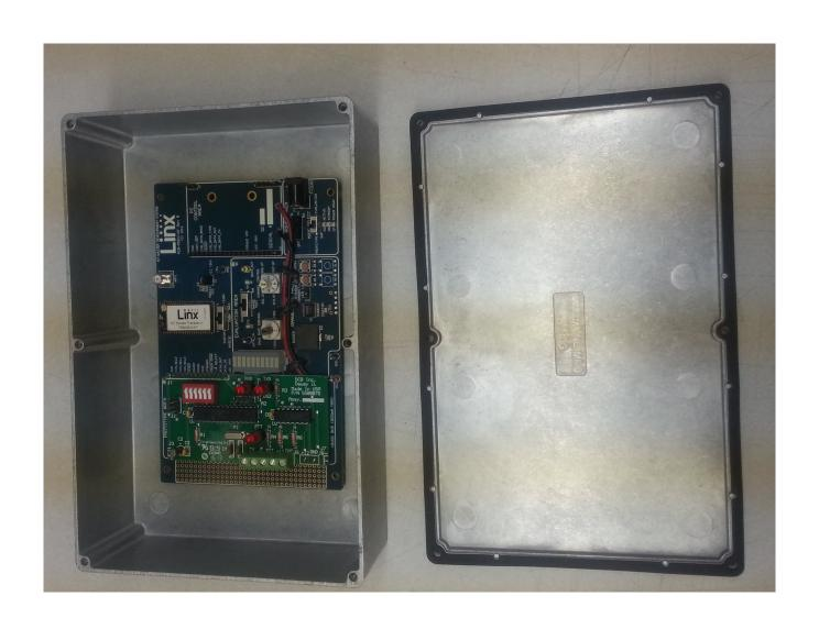
The LX1 radio is asynchronous, serial RS232. It accepts continuous serial data without regard to stop or start bits. It has been designed transport any asynchronous serial RS232 data stream, including asynchronous HDLC protocol. Switch number 4 can be used to squelch or open the receiver of a unit based upon the receipt of 7E HDLC flags.
