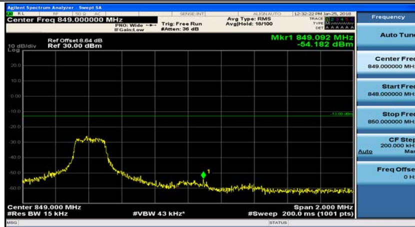
Channel Bandwidth: 10 MHz_HCH_16QAM_1RB#24
