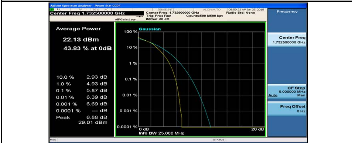
Channel Bandwidth: 10 MHz_MCH_16QAM_50RB#0
