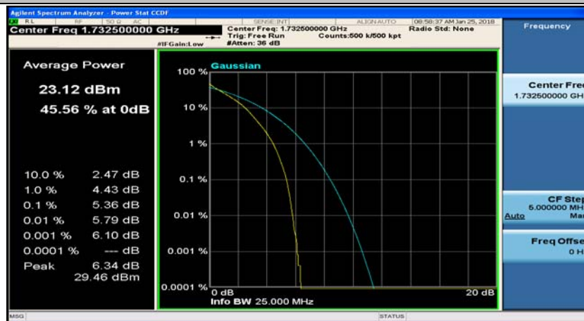
Channel Bandwidth: 10 MHz_MCH_QPSK_25RB#12
