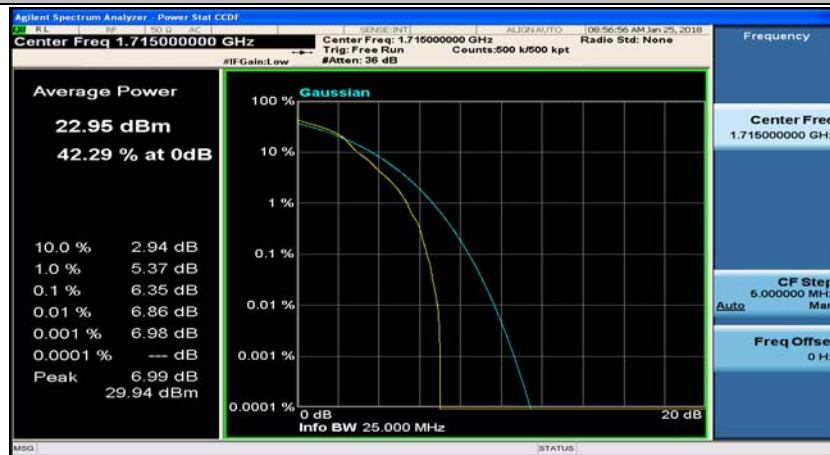
Channel Bandwidth: 10 MHz_LCH_16QAM_25RB#0
