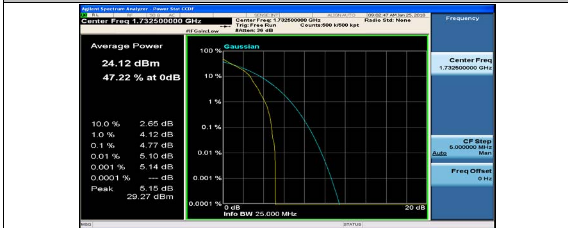
(Channel Bandwidth:15 MHz)_MCH_QPSK_1RB#74
