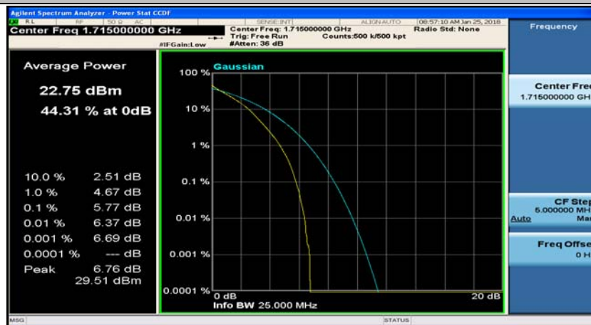
Channel Bandwidth: 10 MHz_LCH_QPSK_25RB#25
