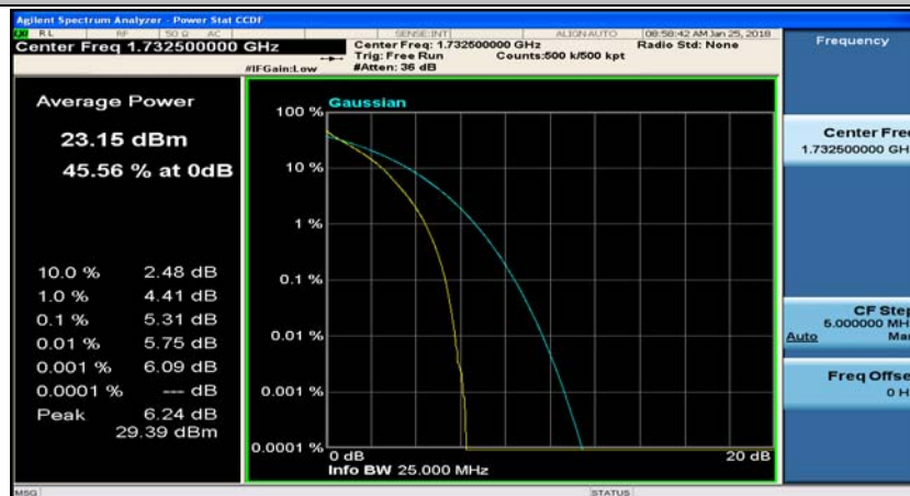
Channel Bandwidth: 10 MHz_MCH_QPSK_25RB#25
