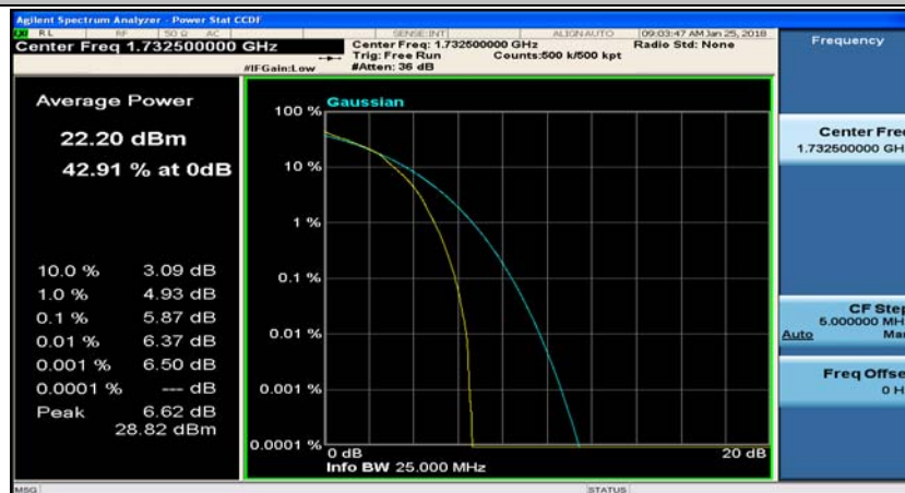
(Channel Bandwidth:15 MHz)_MCH_16QAM_37RB#38
