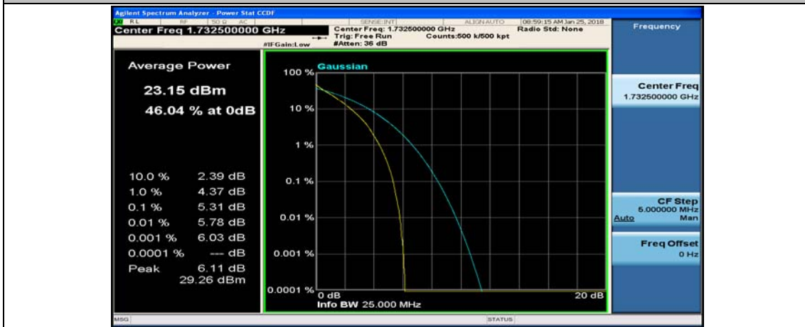
Channel Bandwidth: 10 MHz_MCH_QPSK_50RB#0
