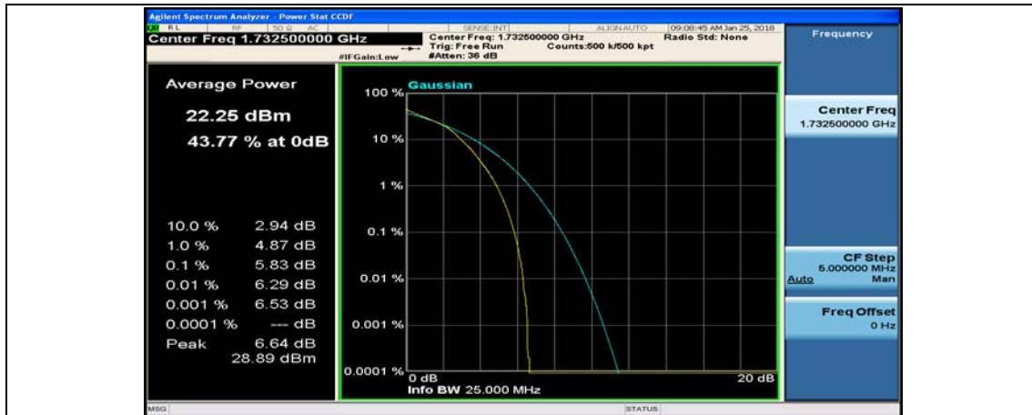
(Channel Bandwidth:20 MHz)_MCH_16QAM_100RB#0
