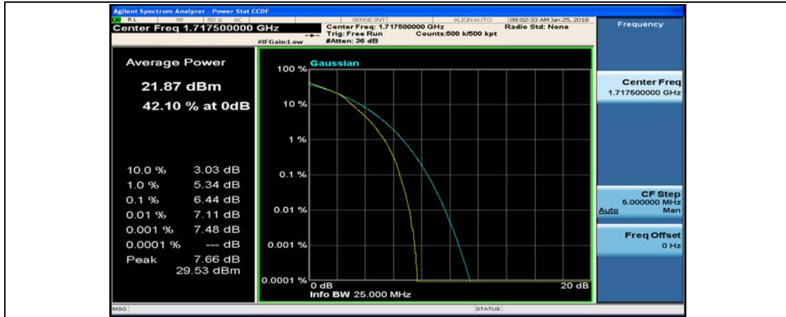
(Channel Bandwidth:15 MHz)_MCH_16QAM_1RB#0
