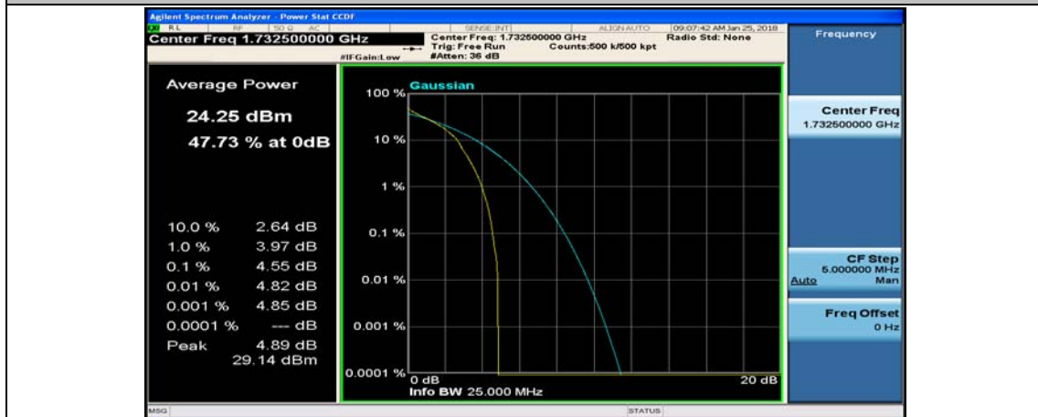
(Channel Bandwidth:20 MHz)_MCH_QPSK_1RB#99
