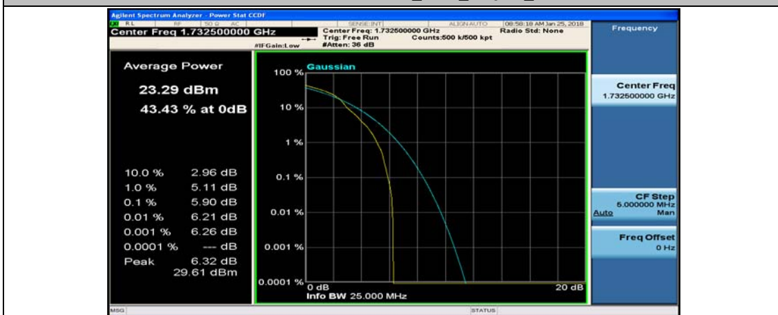
Channel Bandwidth: 10 MHz_MCH_16QAM_1RB#24
