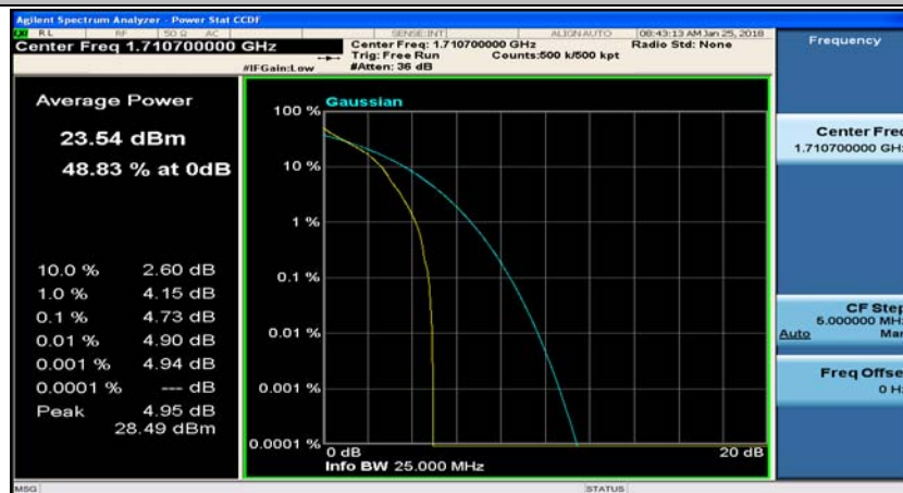
(Channel Bandwidth: 1.4 MHz)_LCH_QPSK_3RB#0
