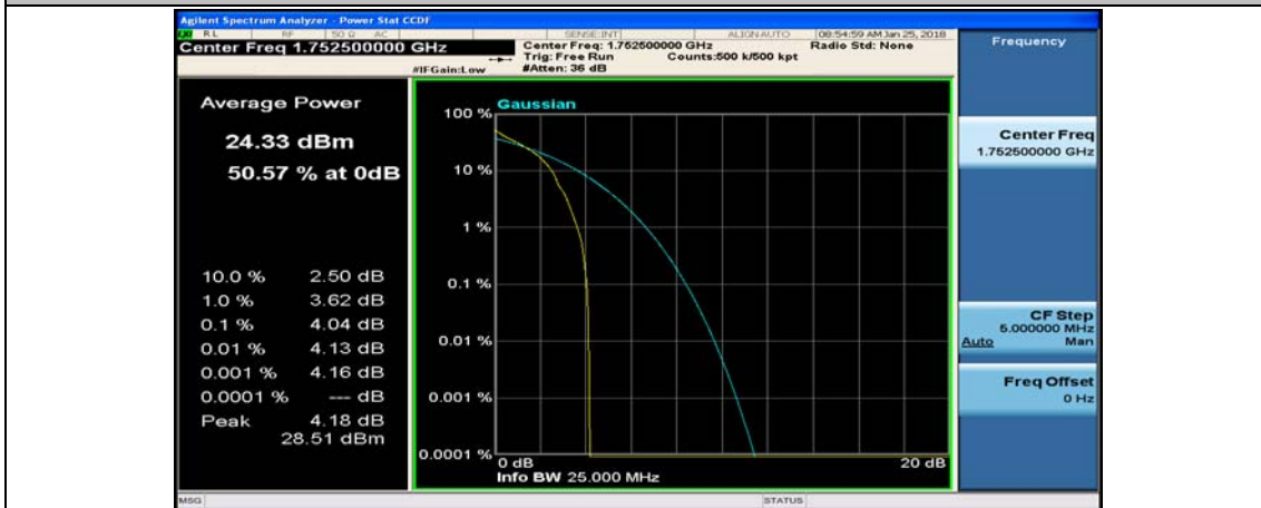
(Channel Bandwidth: 5 MHz)_HCH_QPSK_1RB#12
