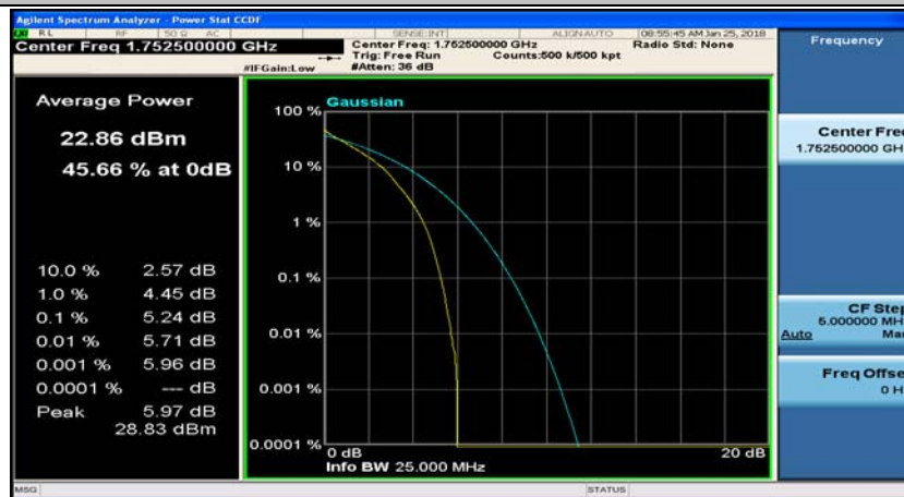
(Channel Bandwidth: 5 MHz)_HCH_QPSK_25RB#0
