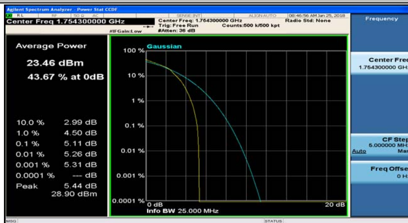
(Channel Bandwidth: 1.4 MHz)_HCH_16QAM_3RB#2
