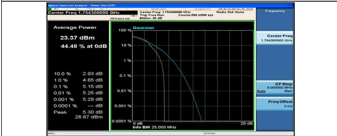
(Channel Bandwidth: 1.4 MHz)_HCH_16QAM_1RB#3
