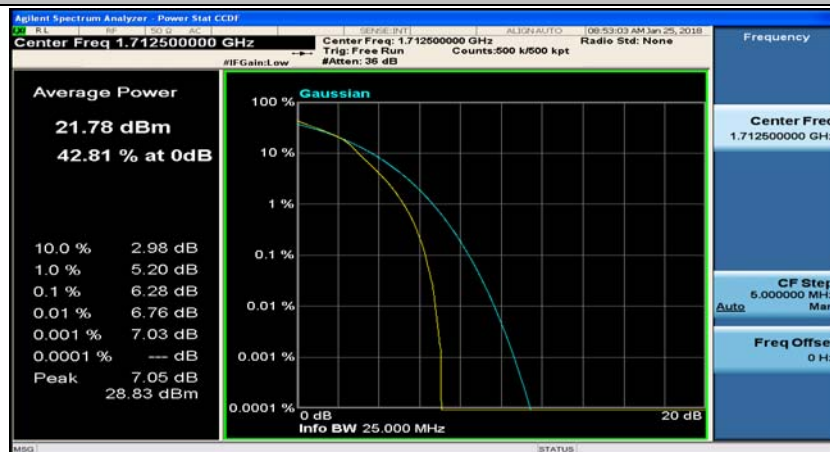
(Channel Bandwidth: 5 MHz)_LCH_16QAM_25RB#0
