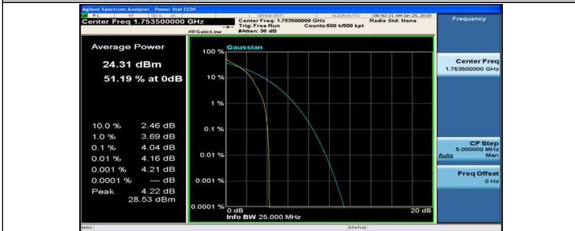
(Channel Bandwidth: 3 MHz)_HCH_QPSK_1RB#7
