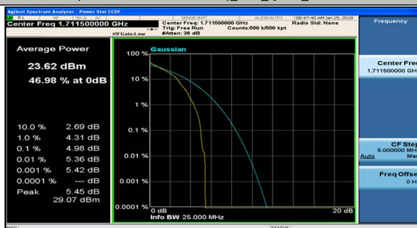
(Channel Bandwidth: 3 MHz)_LCH_QPSK_8RB#0
