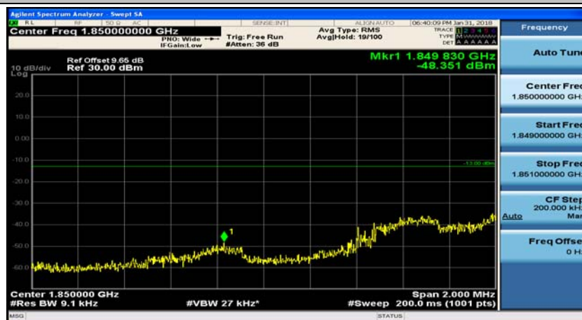
(Channel Bandwidth: 3 MHz)_LCH_16QAM_1RB#14
