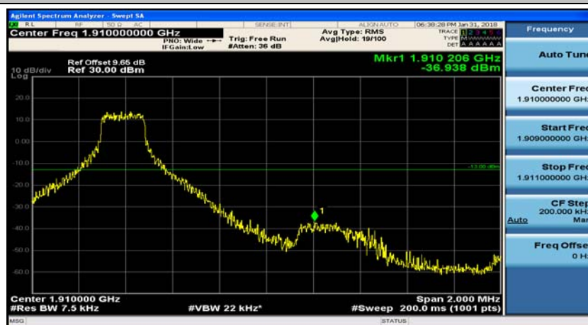
(Channel Bandwidth: 1.4 MHz)_HCH_16QAM_1RB#5
