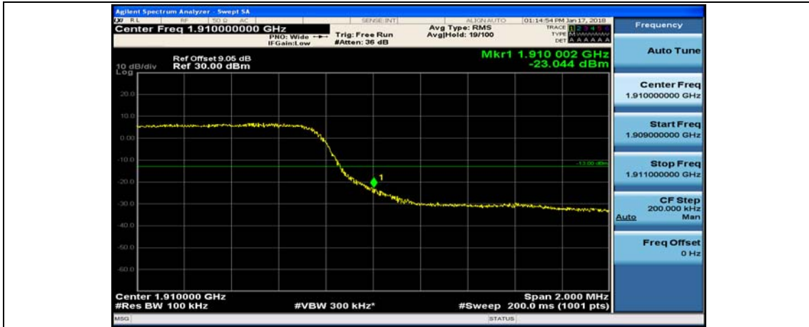
(Channel Bandwidth: 5 MHz)_LCH_16QAM_1RB#0
