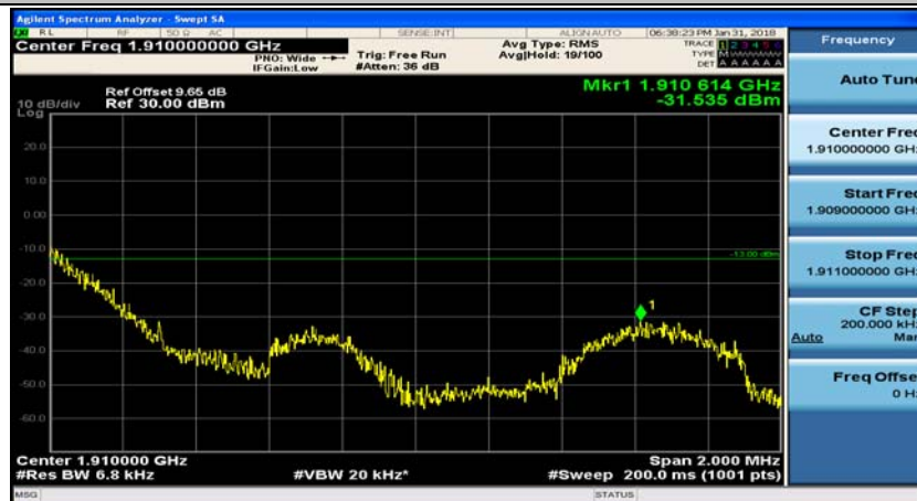
(Channel Bandwidth: 1.4 MHz)_HCH_16QAM_1RB#3
