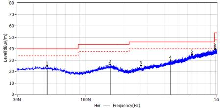
Frequency Reading Factor Level Limit Margin No. Detector Polar MHz dBuV dB/m dBuV/m dΒ dBuV/m 1\* QΡ 50.734 4.20 20.59 24.79 40.00 -15.21 Hor 2\* QP 154.160 4.89 21.56 26.45 43.50 -17.05 Hor 3\* 263.285 5.27 19.98 25.25 46.00 -20.75 QΡ Hor 4\* QP 442.735 4.26 25.83 30.09 46.00 -15.91 Hor QP 5\* 644.859 46.00 5.27 29.83 35.10 -10.90 Hor 6\* 970.415 5.98 33.54 39.52 54.00 -14.48 QΡ Hor
