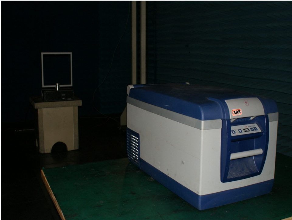
Photograph 2: Set-up for Spurious Emissions (30MHz-1GHz)
