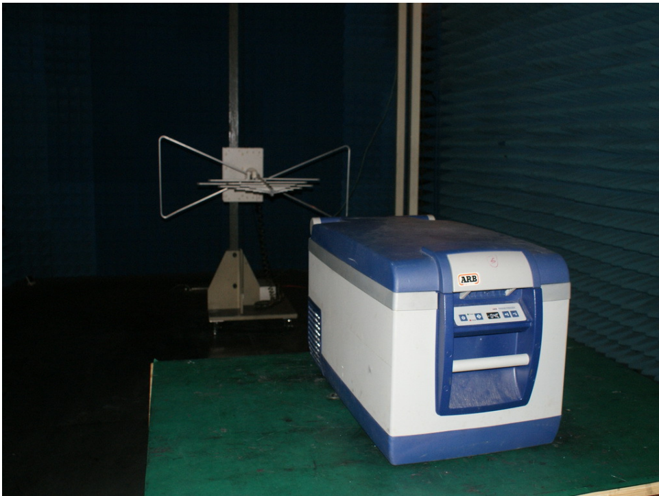
Photograph 2: Set-up for Spurious Emissions (30MHz-1GHz)
