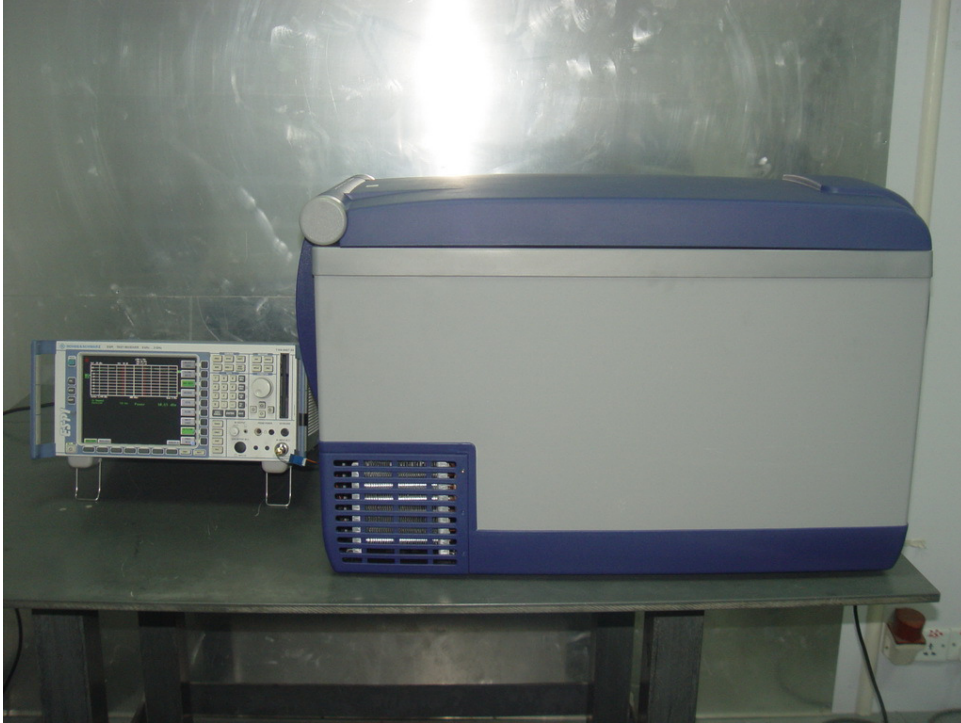
Photograph 5: Set-up for Conducted Emissions
