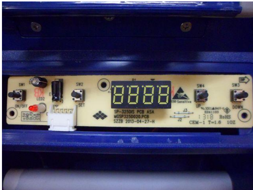
Fig. 3: Internal view of control panel
