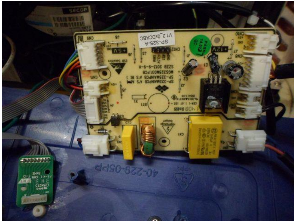
Fig. 1: Internal view of main board
