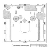
Since the fastening clips of the inductors extend out of the bottom side of the mounting plate, these cannot be placed over certain areas of the generator. For example, certain components of the filter are blocked because they contain air and leakage paths and by the frame of the housing.
