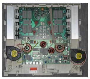
The generator contains up to four frequency converters, a control unit and safety unit, as well as a cooling unit. In addition, it contains the connection for the main supply, relay for separating the converter from the supply voltage, the necessary filters and the small voltage supply of the UI and the bus for communication between user interface and generator.
