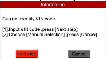
In case the IFIX-430 series diagnostic scanner provides an option for vehicle VIN scan allowing users to input the VIN manually.
