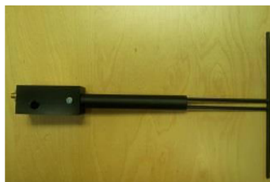
Figure 1 – MVG COMOSAR Validation Dipole
