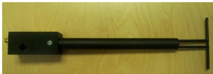
Figure 1 – MVG COMOSAR Validation Dipole
