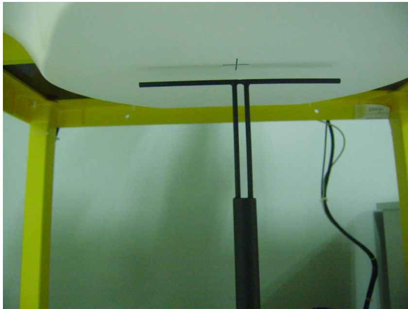
Setup Photo of Dipole Antenna
