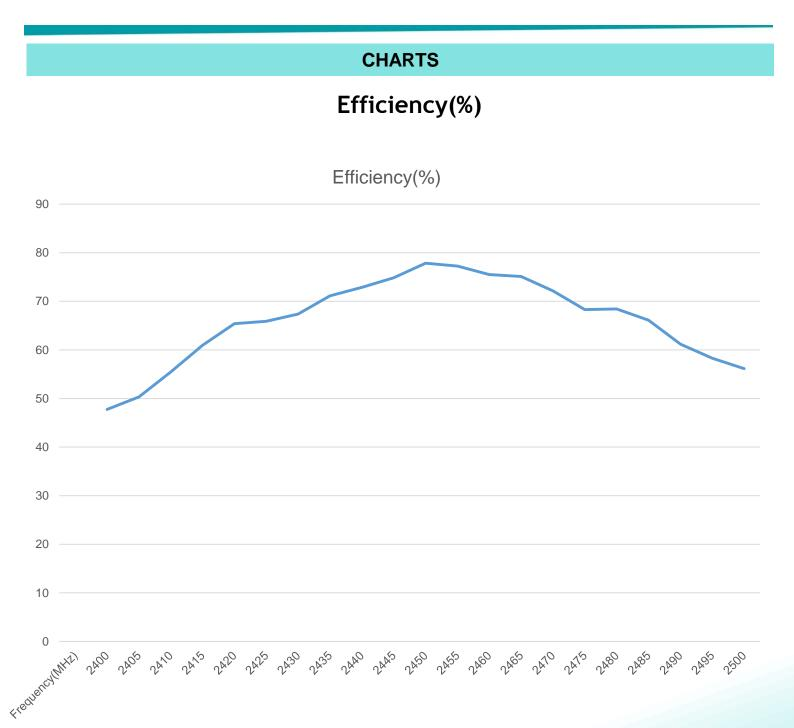
(\*) All RF parameters measured on 80\*37mm PCB with 4\*4.25mm clearance in free space. No matching component used.
