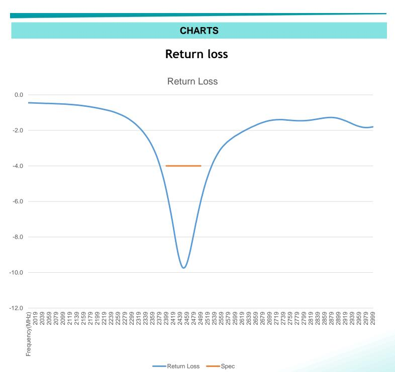
(\*) All RF parameters measured on 80\*37mm PCB with 4\*4.25mm clearance in free space. No matching component used.
