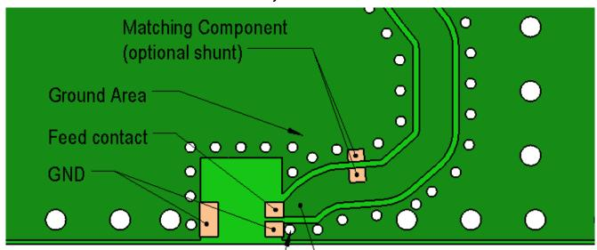
Ground Via Hole Ground area should be surround with ground via holes
