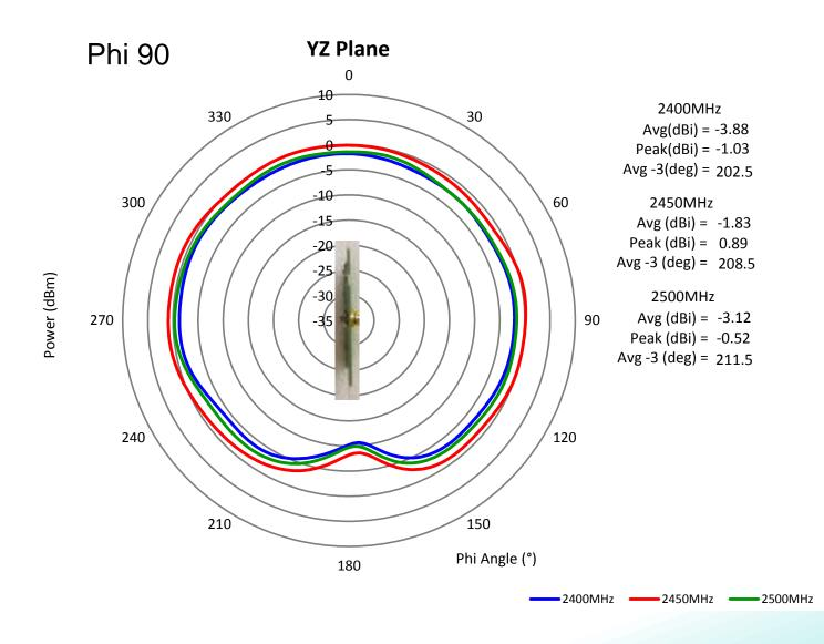
(\*) All RF parameters measured on 80\*37mm PCB with 4\*4.25mm clearance in free space. No matching component used.
