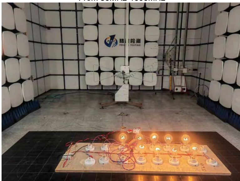
Radiated Spurious Emissions From 30MHz-1000MHz
