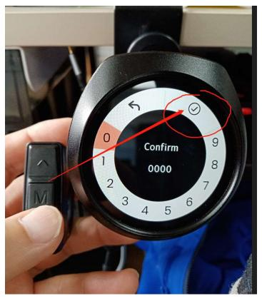
By navigating the UP or DOWN button and locate the orange mark on the "circle tick" then press "M" button to confirm the password setting.
