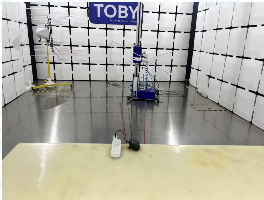
Photo of Setup for Radiated Emission (30MHz~1GHz)
