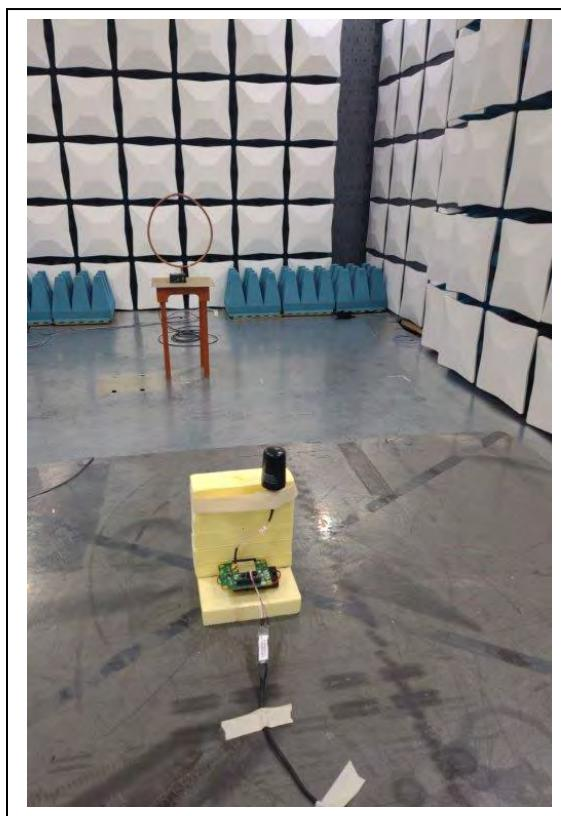
**Radiated Spurious Emissions: 30 MHz to 1000 MHz**
