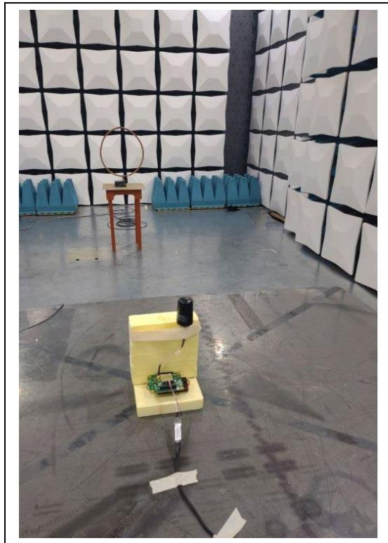
**Radiated Spurious Emissions: Less Than 1 GHz**
