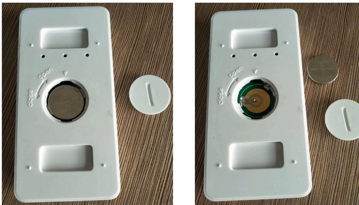
3. Put new battery in the remote, Cover the battery cover.
