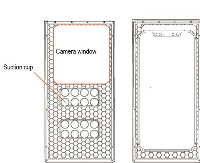
5. Put the inner plate combined with the mobile phone into the diving case. Make sure the handle strap is appressed with the inner plate and not beyond the edge of diving
