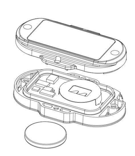
4. When installing a new battery, pay attention to the direction of the battery, with the flat surface facing up (Reference picture identification)
