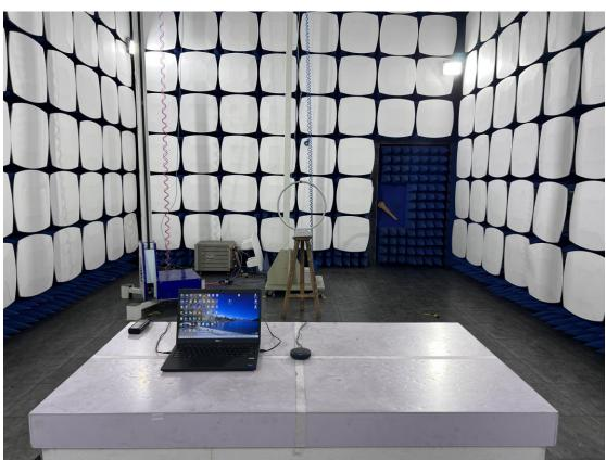
3. Radiated emission (9KHz-30MHz)
