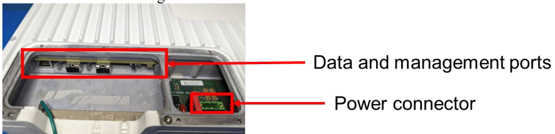
Figure 14 User Accessible Interface Location
