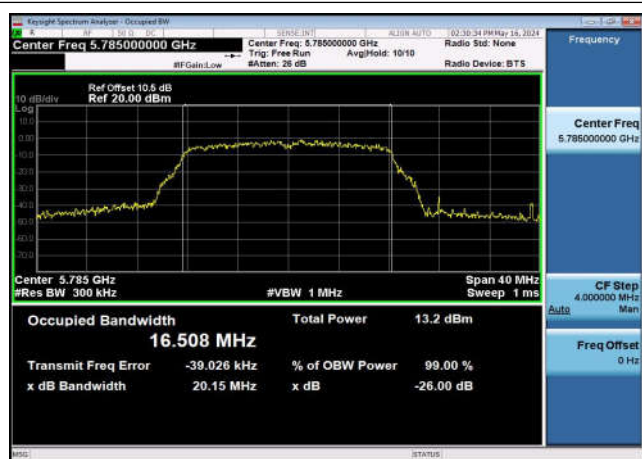
U-NII-3 99%&26dB Bandwidth-802.11ac(20MHz) ,5745MHz,Ant1
