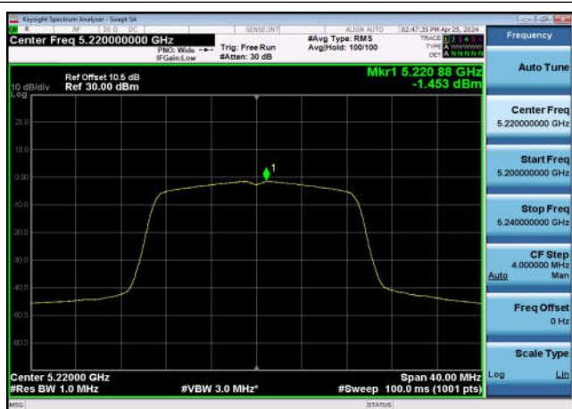
U-NII-1 Power spectral density-802.11 ac(40MHz),5190MHz,Ant1
