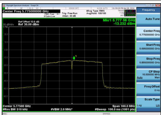
U-NII-3 Power spectral density-802.11 ac(80MHz),5775MHz,Ant1
