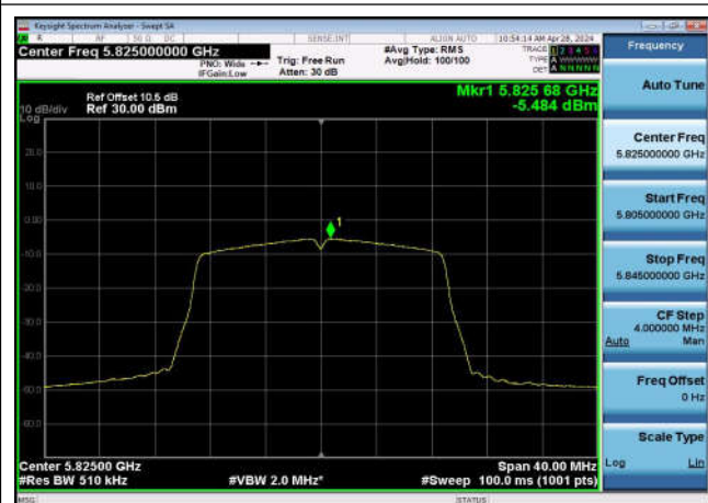
U-NII-3 Power spectral density-802.11 ac(40MHz),5795MHz,Ant1
