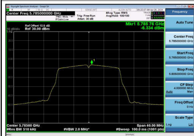
U-NII-3 Power spectral density-802.11 ac(20MHz),5745MHz,Ant1
