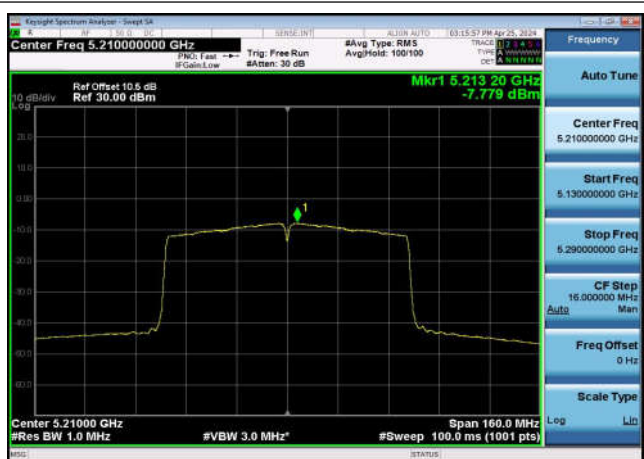
U-NII-3 Power spectral density-802.11 n(20MHz),5785MHz,Ant1
