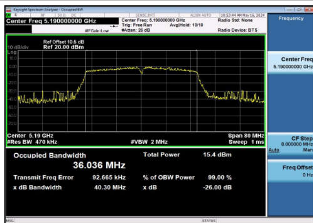
U-NII-1 99%&26dB Bandwidth-802.11a(20MHz) ,5180MHz,Ant1
