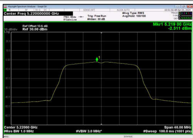
U-NII-1 Power spectral density-802.11 ac(20MHz),5180MHz,Ant1
