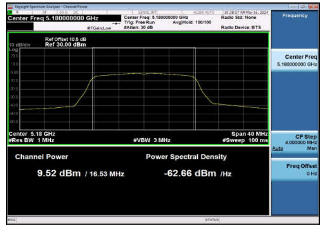
U-NII-1 Output Power-802.11a(20MHz) ,5180MHz,Ant1
