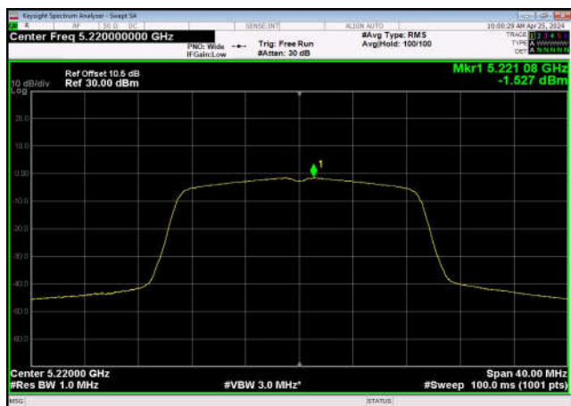
U-NII-1 Power spectral density-802.11 n(40MHz),5190MHz,Ant1
