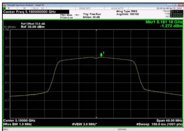
U-NII-1 Power spectral density-802.11 n(20MHz),5240MHz,Ant1
