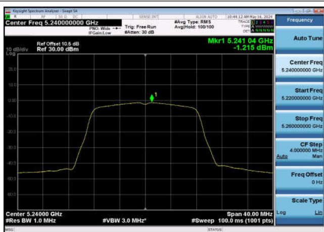
U-NII-1 Power spectral density-802.11 ac(20MHz),5220MHz,Ant1
