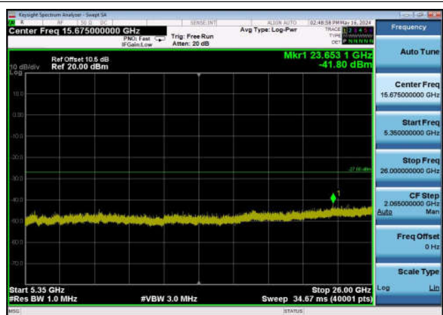
U-NII-1 ,Plot 3,5350MHz~26000MHz-802.11a(20MHz),5240MHz,Ant1
