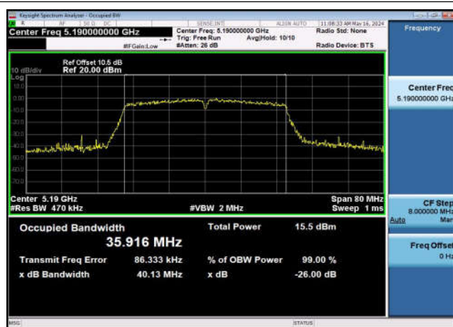
U-NII-1 99%&26dB Bandwidth-802.11ac(40MHz) ,5190MHz,Ant1
