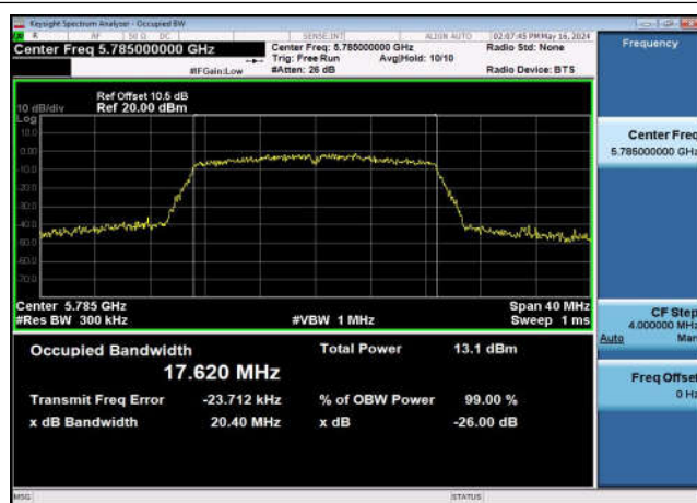
U-NII-3 99%&26dB Bandwidth-802.11ac(20MHz) ,5785MHz,Ant1
