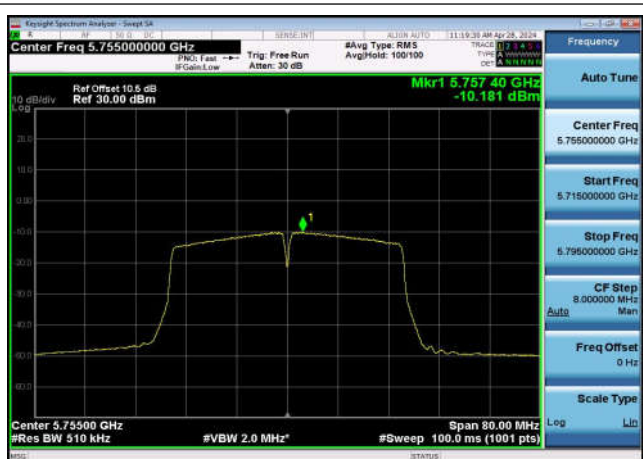
U-NII-3 Power spectral density-802.11 ac(80MHz),5775MHz,Ant1
