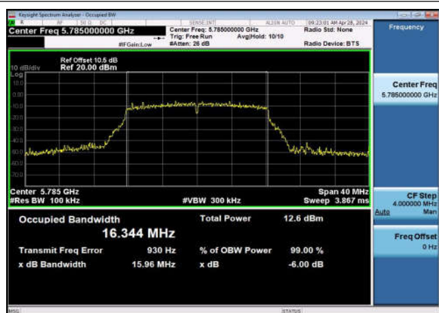
U-NII-3 6dB Bandwidth-802.11ac(20MHz) ,5745MHz,Ant1
