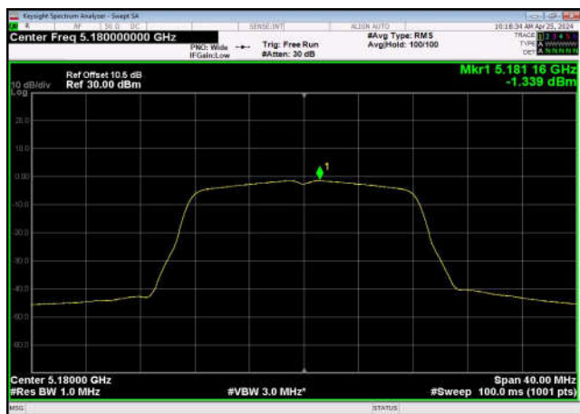
U-NII-1 Power spectral density-802.11 a(20MHz),5180MHz,Ant1
